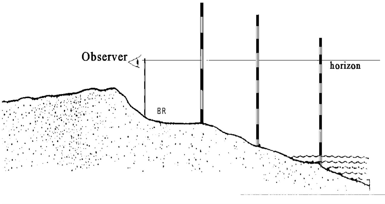
Figure 5. Beach profiling by an observer sighting the horizon from a fixed point.
