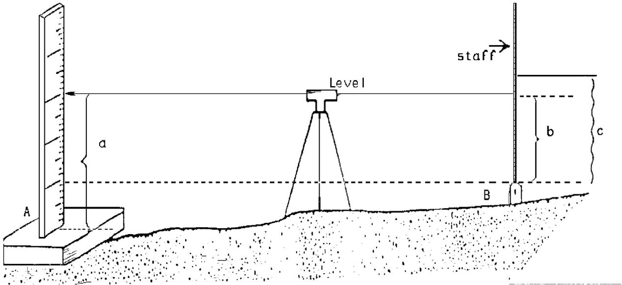
Figure 4. Beach profiling with the aid of a surveyor's level.
