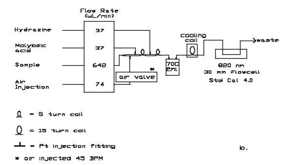
Figure 8.2.b Flow diagrams for the phosphate method. b. OSU RFA method. See text for wavelength considerations. BPM signifies bubbles per minute.
