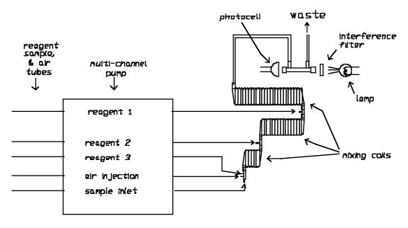
Figure 8.1. A generalized continuous flow analyzer, schematic picture.
