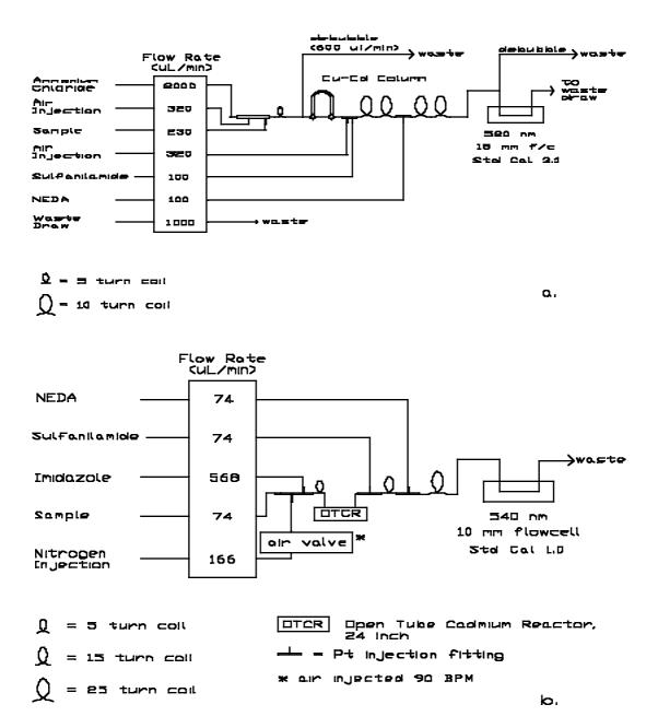
Figure 8.3. Flow diagrams for the nitrate method. a. AA-II. b. RFA See text for discussion of wavelengths. "ul/min" signifies  $\mu$ l/min.
