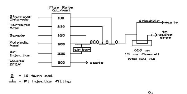
Figure 8.6.a. Flow diagrams for the silicic acid method. (a)AA-II. See text fot wavelength considerations, also for differing paramets at OSU and SIO-ODF.
