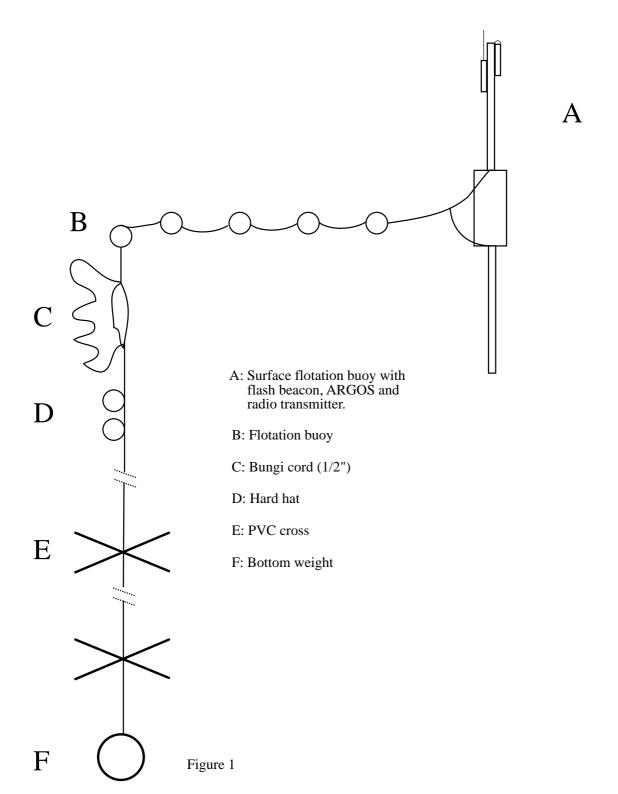
Figure 25.1. The surface-tethered trap array.
