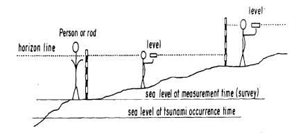
hand carpenter's level or by "reading" the intersection height of the sea/sky horizon line with the rod (or companion person) standing at the sea level shore-line. Leap-frogging by subsequently re-positioning the rod at the so positioned points, and the observer at new upper unknown ones, until the highest water mark is reached, its elevation will be determined. See Figure below (adapted from Japanese Meteorological Organization, 1990).
