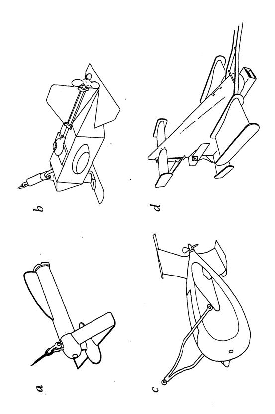
Figure 3. Towed bodies for plankton samplers. a - plankton indicator; b - continuous plankton recorder; c - undulating oceanographic recorder; d - Batfish.
