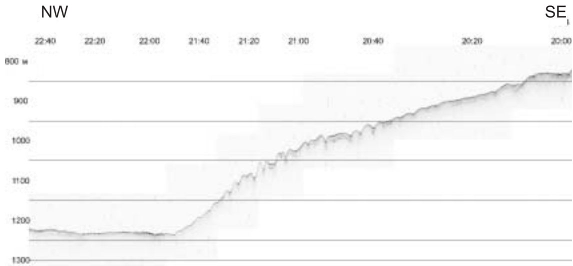
Figure 49. 5 kHz sediment profile along Line PSAT-206 showing contourite mud waves and basin floor.
