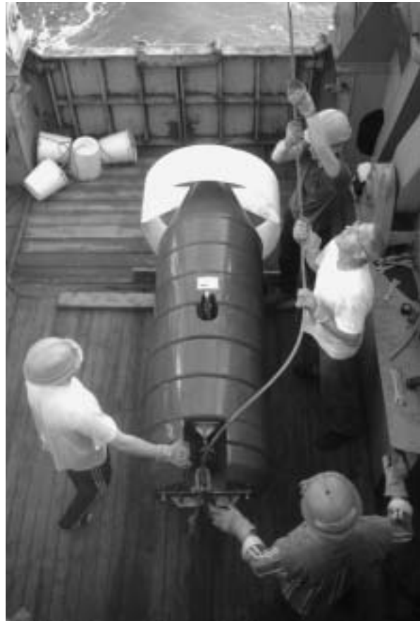
MAK-1M sidescan sonar system: preparation for deployment
