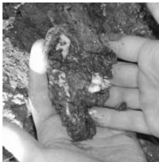
Figure 14. Gas hydrates in the Core BS308K.
