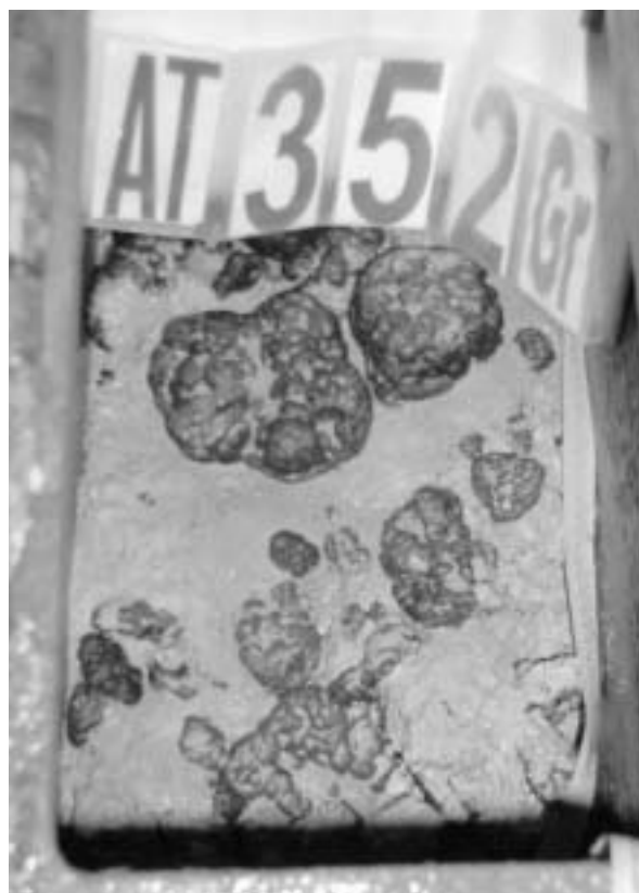
Figure 75. Polimetallic crusts sampled at station AT-352GR.
