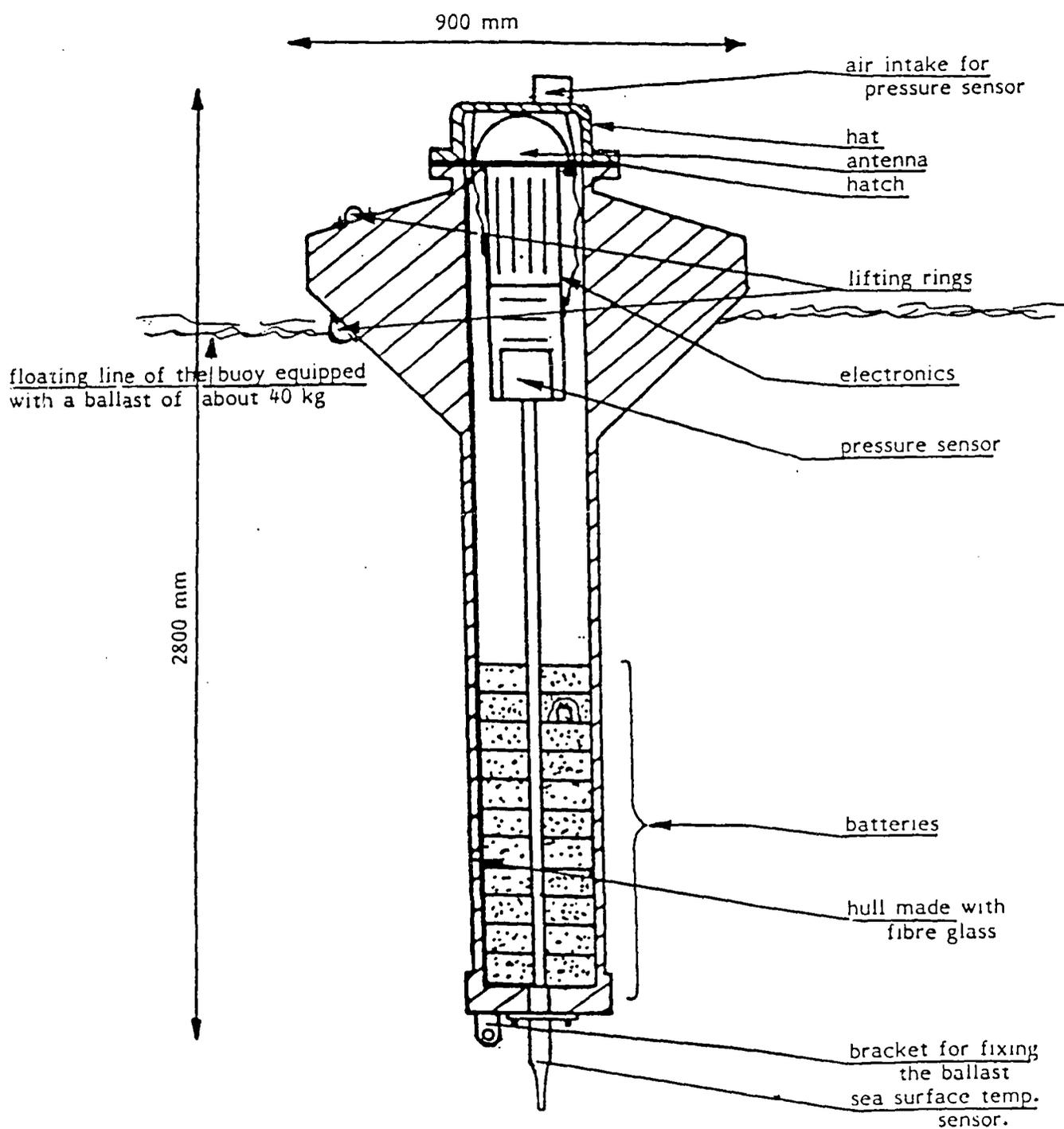
Prototype of Marisonde BT with sub-surface temperature chain
