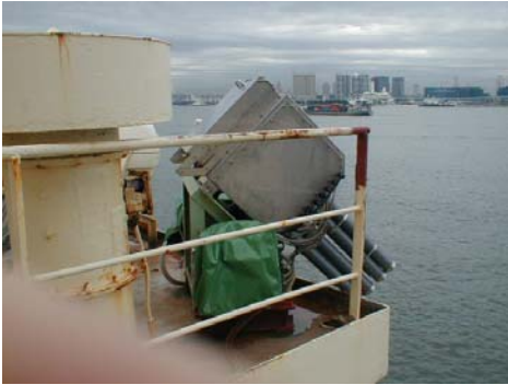
Photo 1. Automated XBT/XCTD launcher
