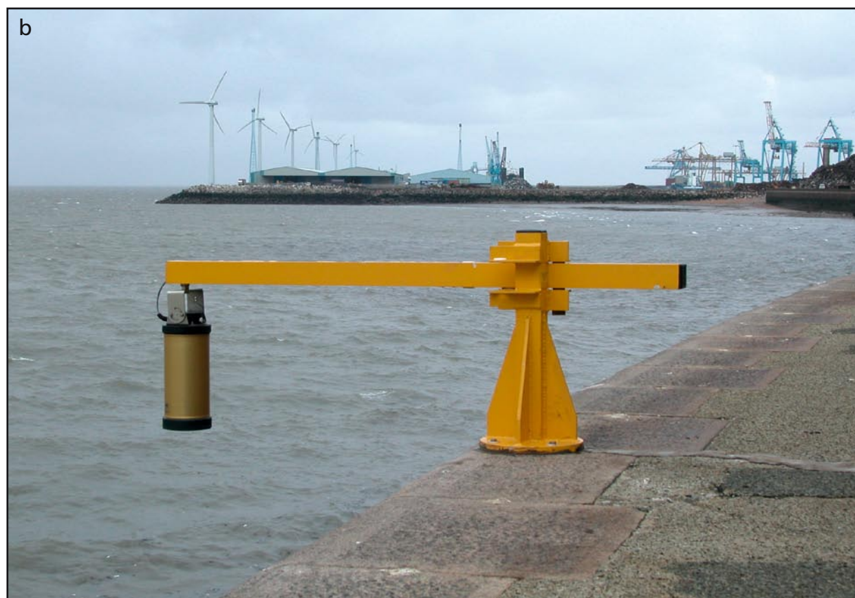
Figure 3.6 Radar tide gauges.
