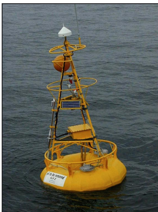
Figure 8.3 The GFZ Potsdam GPS buoy.
