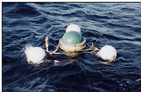
Figure 8.1 The University of Tasmania GPS buoy (C. Watson, personal communication).
