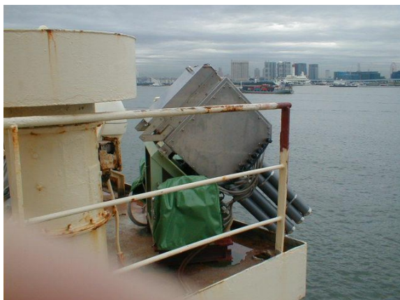
Photo 1. Automated XBT/XCTD launcher
