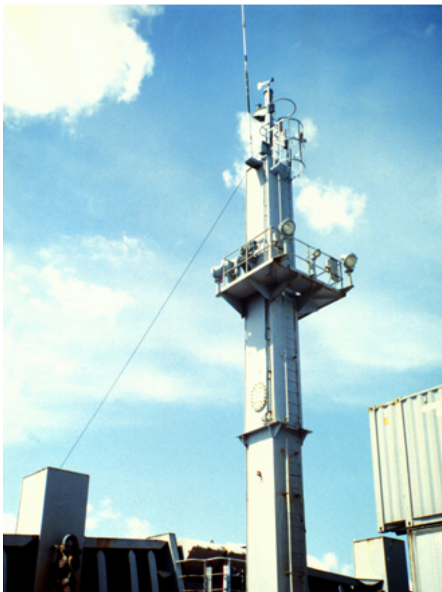
Figure 6 - Bow mast with IMET instruments at top.
