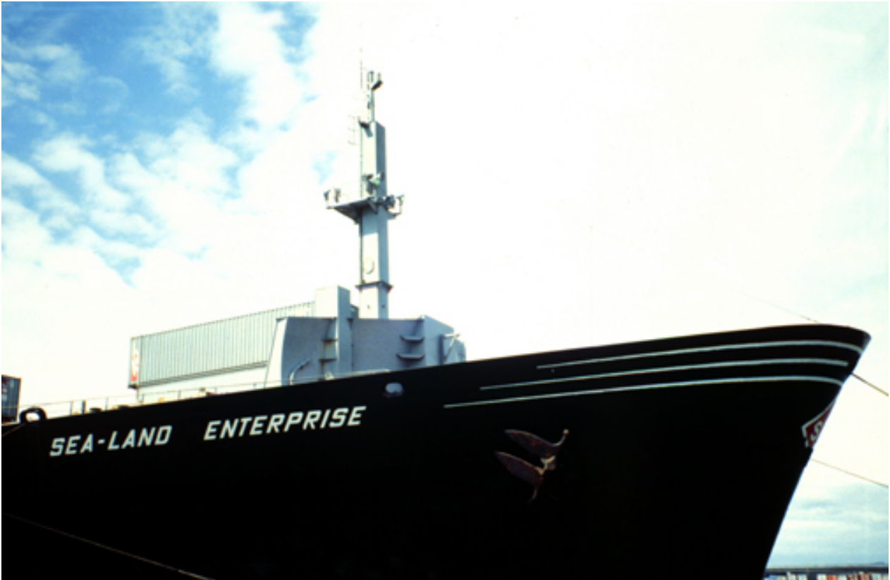
Figure 5 - Bow view of the SeaLand Enterprise. Bow mast with sensors is 70 feet above the deck.
