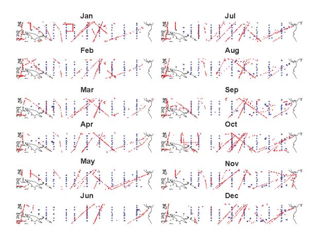
Figure 7. Geographic locations of TAO/TRITON arrays (blue) and other equivalent sources of subsurface thermal observations (red) during 2000.
