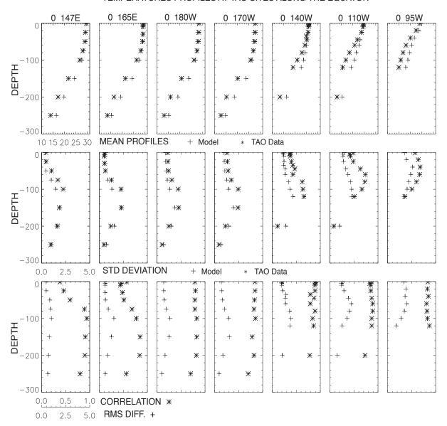
Figure 9. Comparison between model and TAO in situ temperatures along the equator at 147 E, 165 E, 180, 170 W, 140 W, 110 W, and 95 W. The upper panel shows the mean profiles, the middle panel the standard deviation, and the lower panel the rms difference and correlation (from Vialard et al., 2001).
