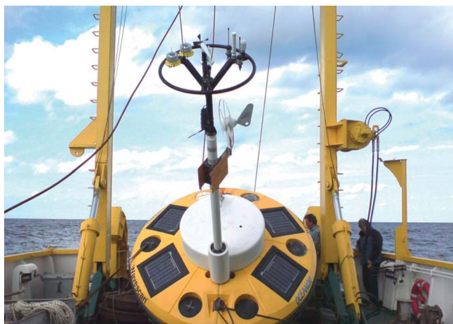
The Poseidon Pylos research time series station ( http://www.euro-sites.info/pylos.php ) is the first (mooring) in the NEAMTWS region with a bottom platform for tsunami detection.
