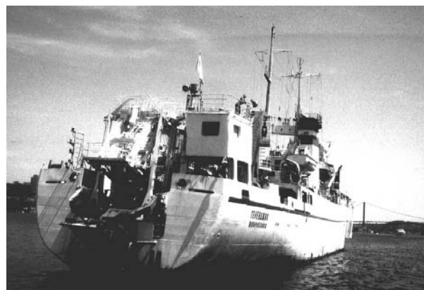
R/V Professor Logachev, the TTR 'floating university' ship: most of its heavy geological and geophysical equipment is operated from a specially designed stern
