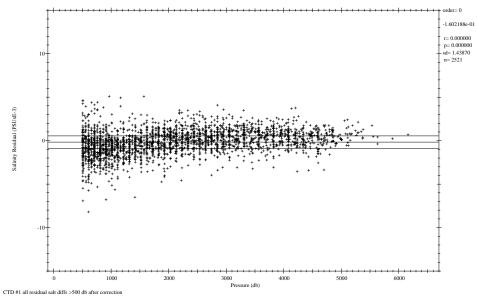
Figure 1.6.3 Salinity residual differences vs pressure (after correction).
