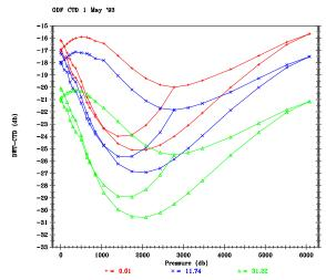
Figure 1.5.0 Pressure calibration for ODF CTD #1, May 1993.
