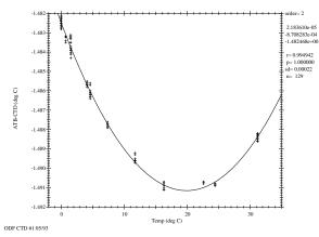
Figure 1.5.3 Temperature calibration for ODF CTD #1, May 1993.
