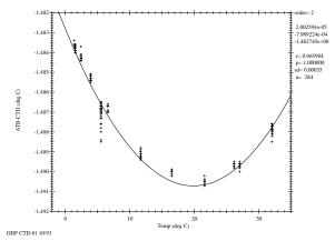
Figure 1.5.4 Temperature calibration for ODF CTD #1, October 1993.
