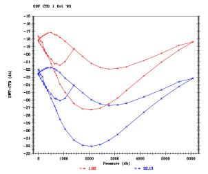
Figure 1.5.1 Pressure calibration for ODF CTD #1, October 1993.
