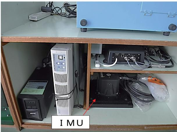
Photo 3. IMU installed at the bottom of the instrument rack of S/V *Kurushima*.
