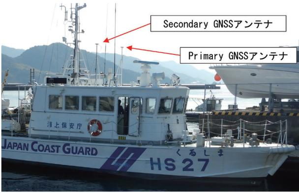
Photo 2. Mast of S/V *Kurushima* equipped with GNSS antennas.
