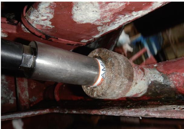
Photo 4. Surface sound speed sensor on the hull of S/V *Kurushima*.
