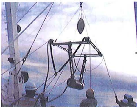
Photo 1 Operation of deploying a 4,000inch 3 airgun.
