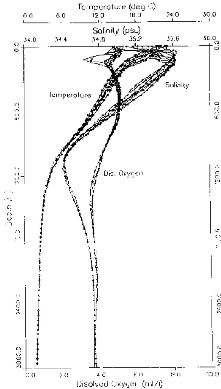
Fig. 9. Example of vertical profiles of temperature, salinity and dissolved oxygen, from the cruise in Fig. 8.
