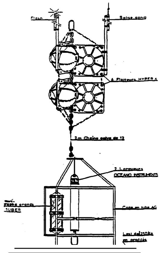
Figure 1b: diagramme of the plateau station with its SUBER pressure gauge and its Oceano-Instruments release device.
