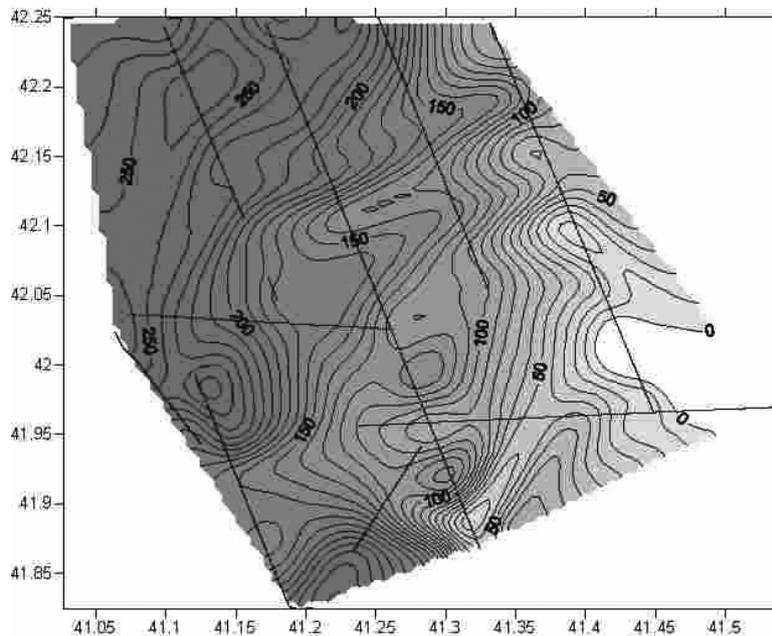
Figure 1. Thickness of gas hydrate stability field
