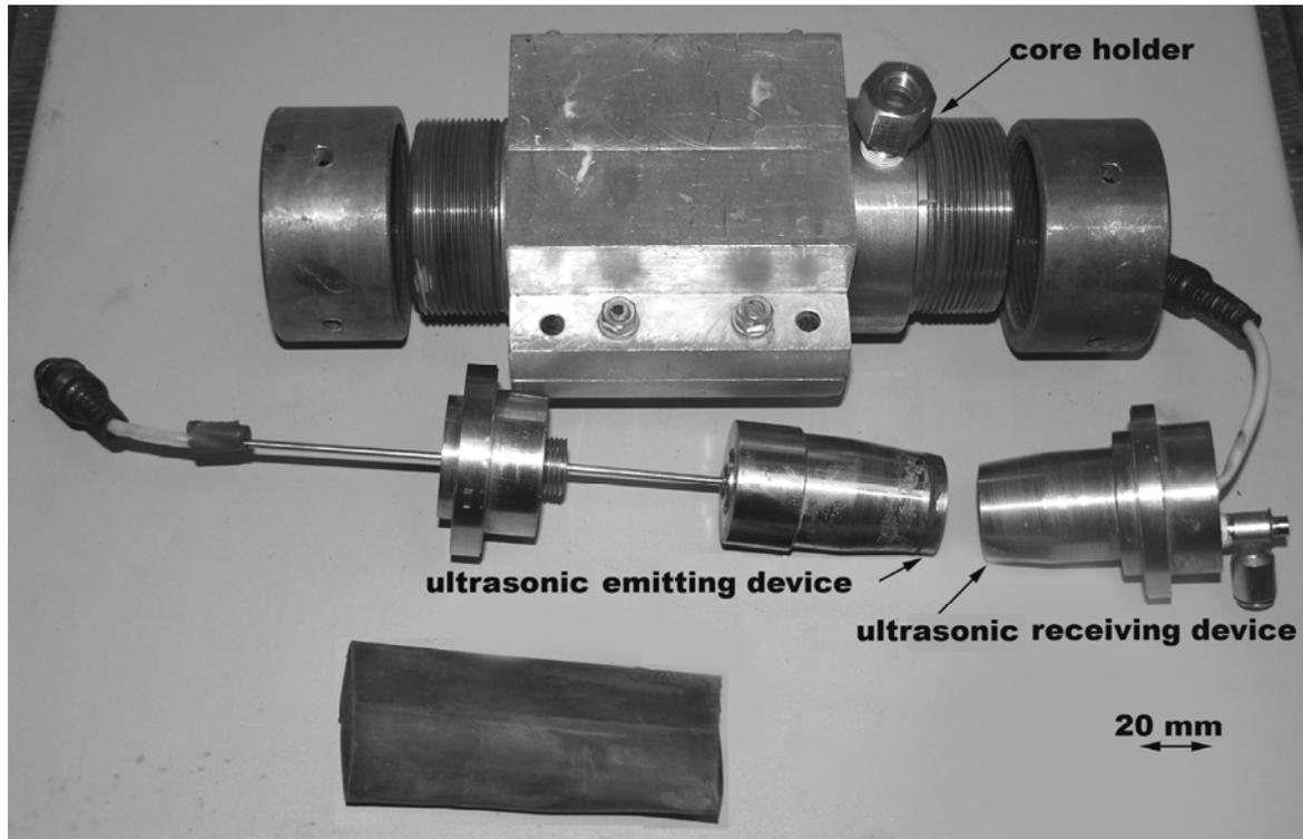
Figure 2. Acoustic measurement block of the PUMA-650 analyser
