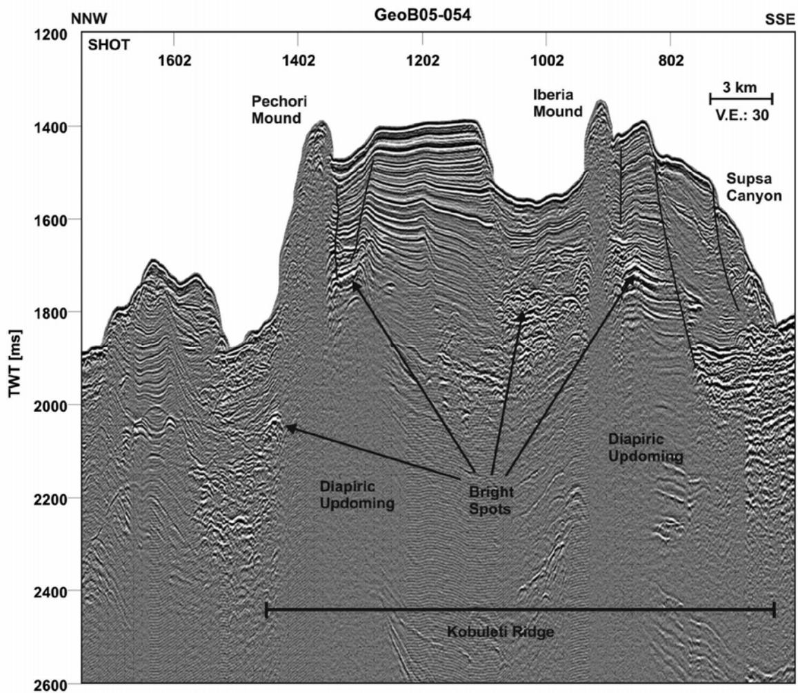
Figure 2. Stacked seismic section GeoB05-054
