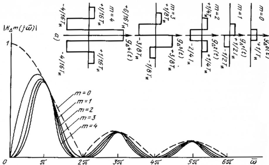
Figure 1. AFC of filter determined by the integrating unwrapping transformation
