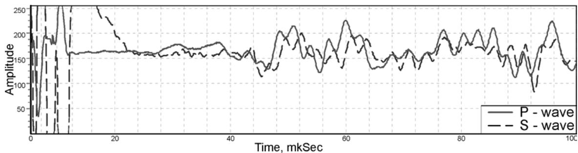
Figure 3. Pattern of P and S waves in the sample of frozen natural gas hydrate bearing sediments
