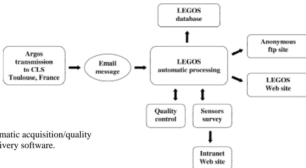
**Figure 3.** Automatic acquisition/quality control/fast-delivery software.
