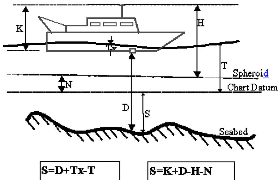
**Figure 1.** Diagram of the Real Time Kinematic GPS (RTK-GPS) system which allows soundings to be reduced in real time without the need for tidal measurements; *spheroid* is the conventional radar altimetric reference surface for measuring sea height.
