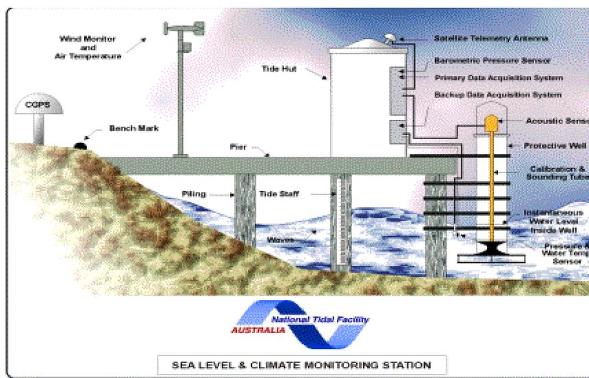
**Figure 1.** Schematic of the SEAFRAME acoustic tide gauge system.
