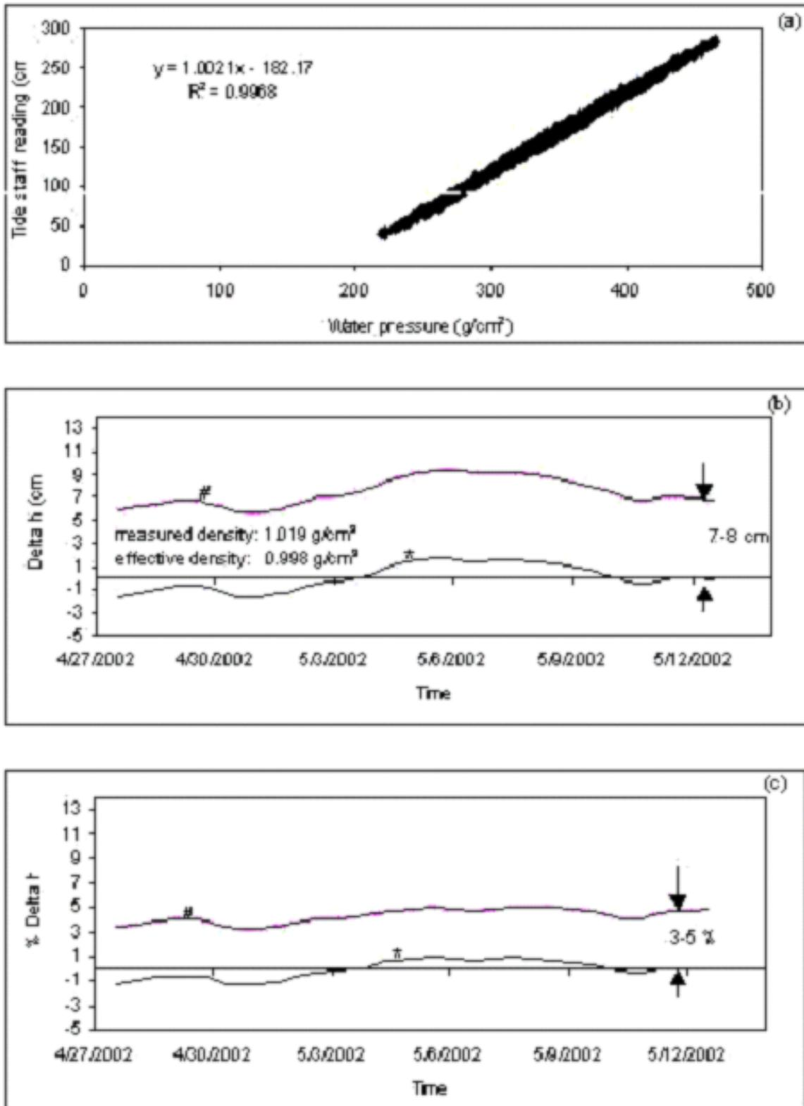
**Figure 11.** (a) Statistical relation based on regression analysis of the entire data set of pressure gauge and tide staff measurements from Kumbarjua Canal site; (b) daily mean difference,  $\Delta h$ , between tide-staff measurement and pressure-derived water level based on measured density (#) and effective density (\*); (c) %  $\Delta h$ .
