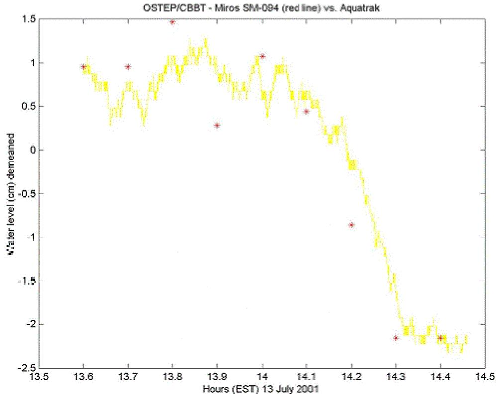
**Figure 1.** Demeaned comparison of Miros SM094 (line) with 6-minute NWLOP water level data (dots).
