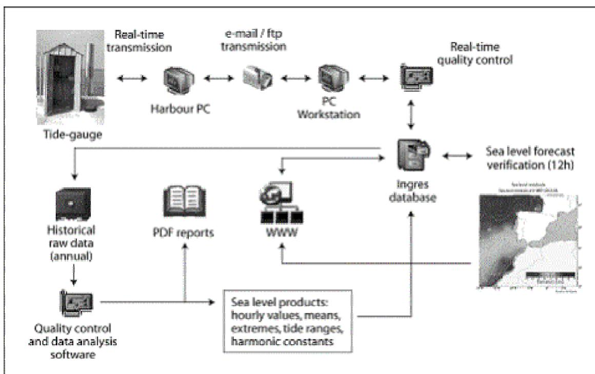
**Figure 1.** Scheme of the flow of sea level data and data processing from a tide gauge station to the web page of Puertos del Estado.
