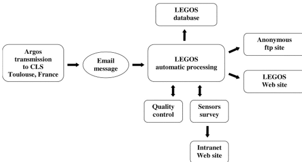
**Figure 3.** Schema of the automatic software presently developed at LEGOS for the ROSAME network.
