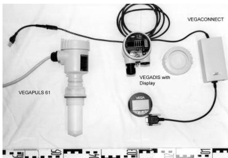
**Figure 2.** Components of the VEGA radar system.
