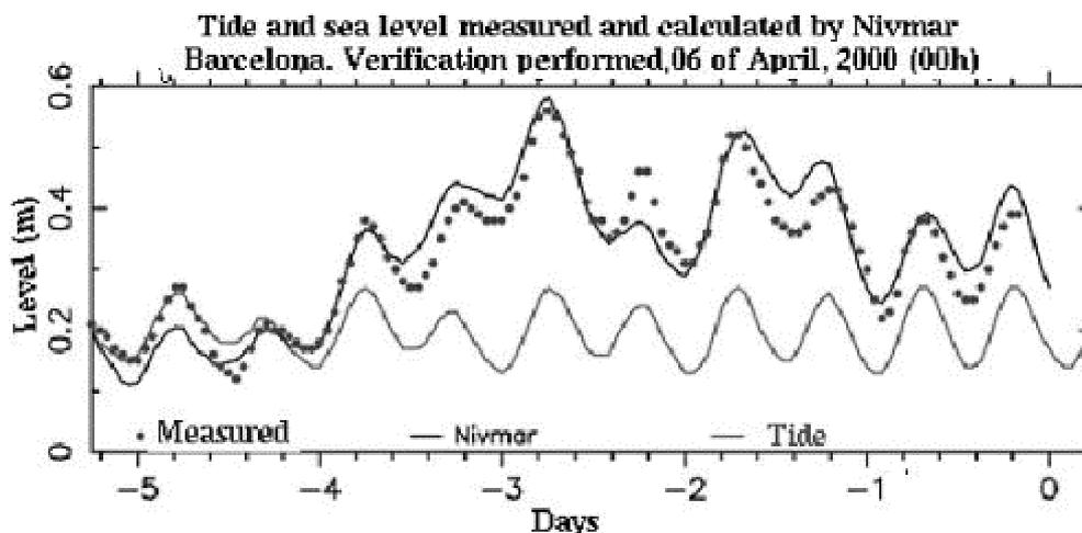
**Figure 2.** Example of validation of the storm surge forecasting system Nivmar with the tide gauge data for the Barcelona tide gauge. The value of 0 on the x-axis corresponds to the initial time of prediction, and comparison is made with the predictions of previous days.
