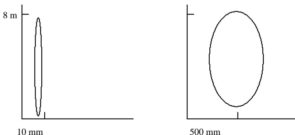
**Figure 2.** Hysteresis in a bubbler system with 1.9-mm tube radius. Tube lengths are 200 m (left) and 1500 m (right).
