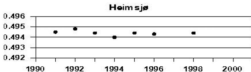
**Figure 3.** Leveling record for the Stavanger (decreasing trend) and Heimsjø (no trend) tide gauges.
