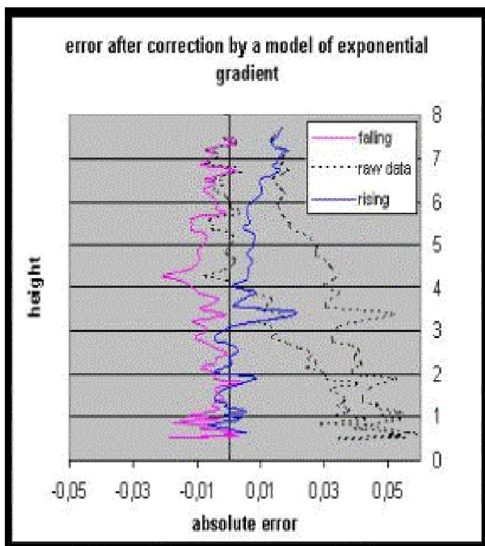
**Figure 6.** Error correction of height measurements using an exponential gradient model.
