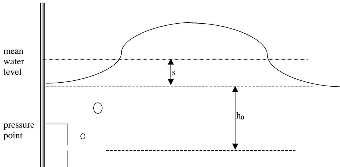
**Figure 3.** Wave parameters for pressure point corrections.
