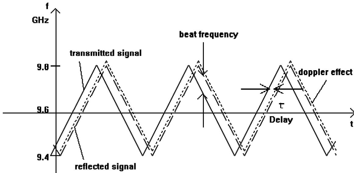
**Figure 2.** Principle of the Miros continuous wave swept frequency.
