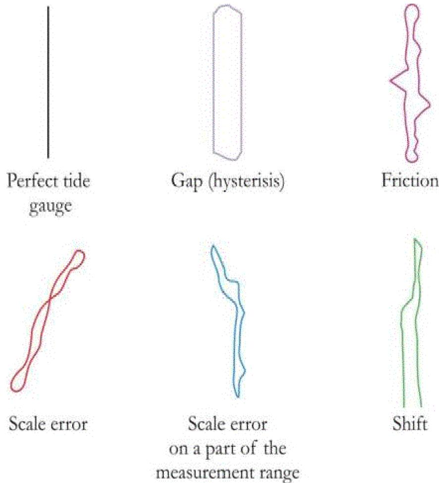
**Figure 1.** Diagram showing the different kinds of typical error highlighted by the VDC test.
