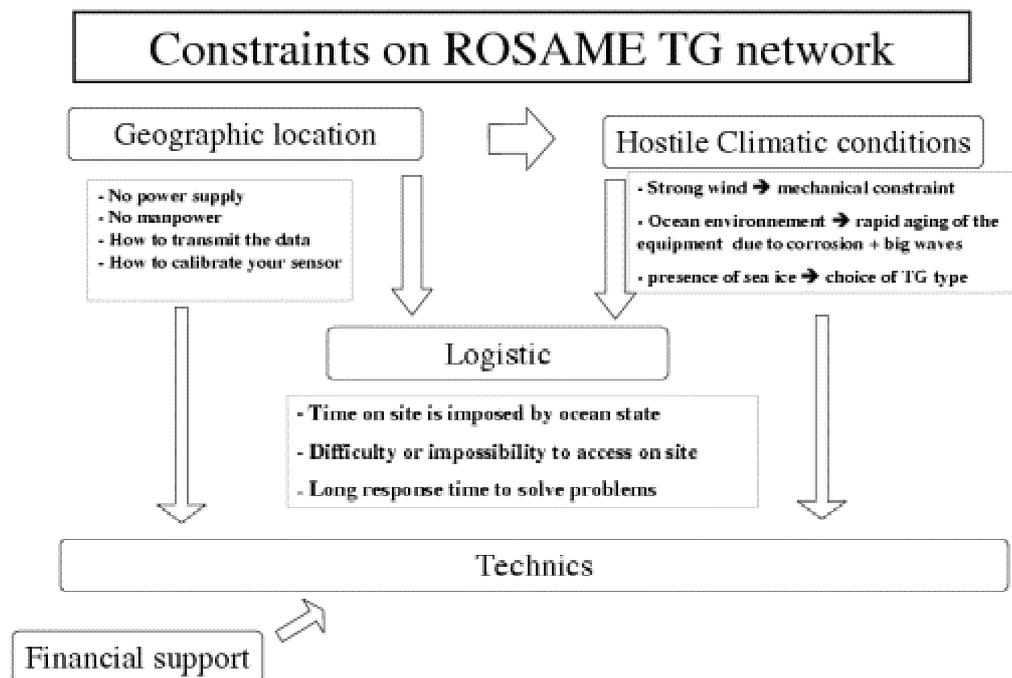
**Figure 3.** Schematic presentation of constraints associated with the ROSAME tide gauge network.
