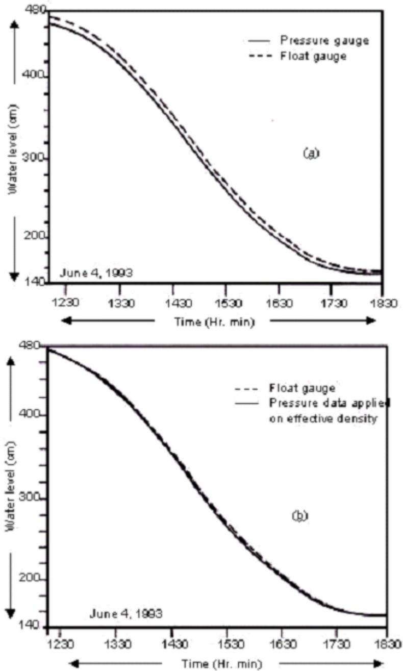
**Figure 6.** (a) Tidal range under-estimation by a pressure gauge deployed in a partially constrained turbid water body of Figure 5 when the measured density of clear water was used for translation of pressure to water elevation; (b) correction of tidal range under-estimation by a pressure gauge deployed in a partially constrained turbid water body of Figure 5 by the application of effective density (After Joseph, 1996).
