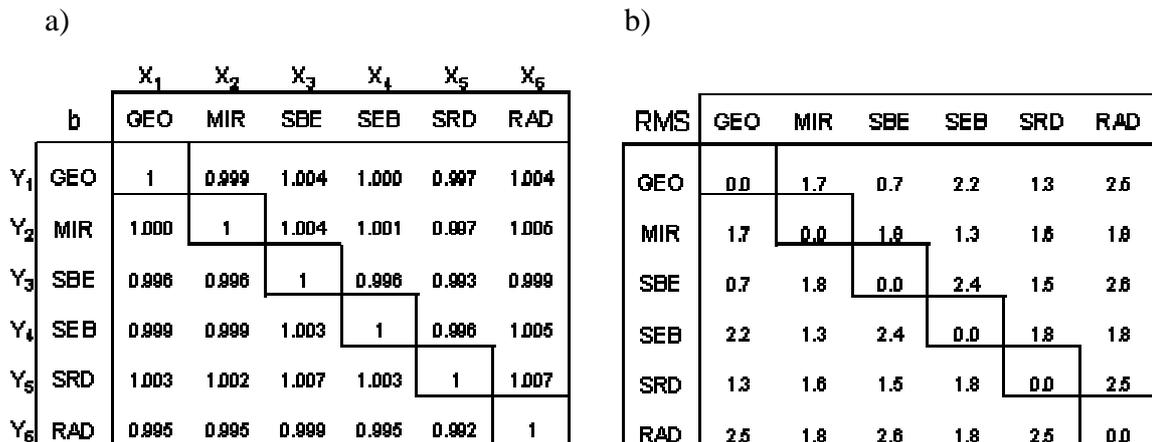
**Figure 6.** Results of the intercomparison between the different gauges in May–June. Slope of the linear regression (a) and RMS (b) (results in centimetres).
