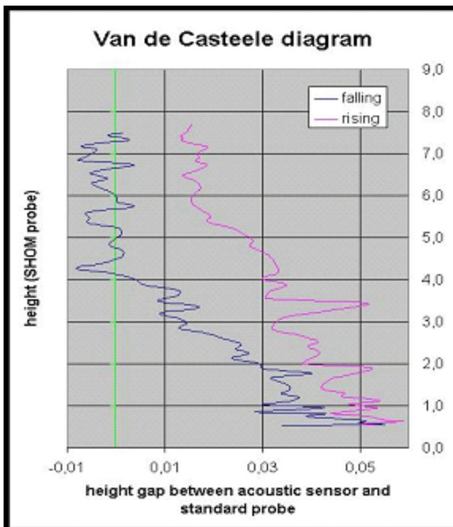
**Figure 3.** Comparison of the SHOM probe and acoustic-sensor (in a stilling well) plots.
