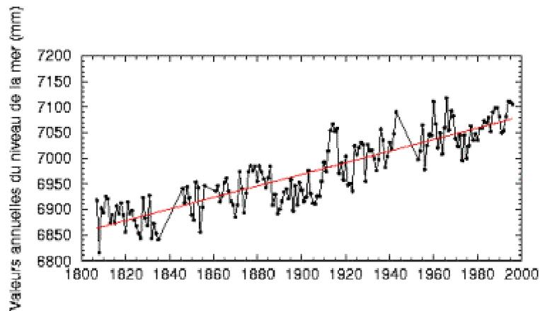
The mean sea level trend is about 1.4 mm/year since the end of the nineteenth century. The absolute-gravity measurements in Brest have been made since 1998 with the French absolute gravity FG5#206 from the EOST (Amalvict et al., 2000).
