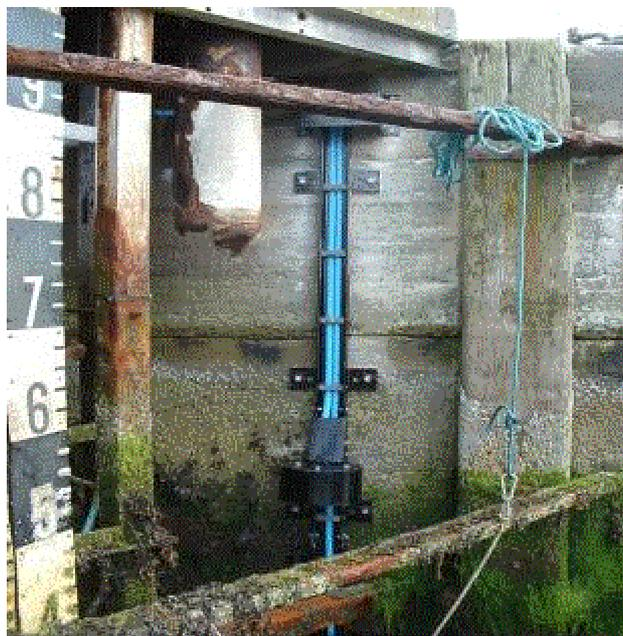
**Figure 4.** The mid-tide pressure point for the bubbler installation at Lerwick, Scotland.
