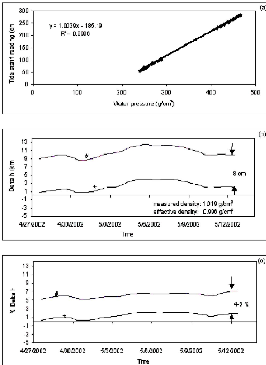
**Figure 10.** (a) Statistical relation based on regression analysis of a small data set of pressure gauge and tide staff measurements from Kumbarjua Canal site, centred on the low and high tide during a spring tide; (b) daily mean difference,  $\Delta h$ , between tide-staff measurement and pressure-derived water level based on measured density (#) and effective density (\*); (c) %  $\Delta h$ .
