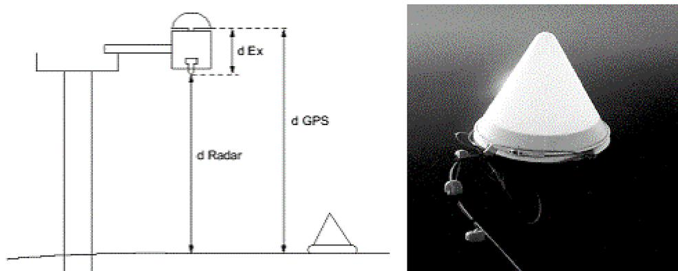
**Figure 7.** Left: principle of the absolute comparison with the GPS buoy; right: GPS buoy.
