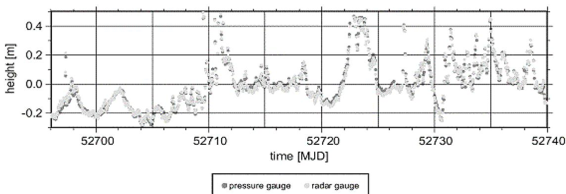
**Figure 5.** Comparison of pressure and radar gauge measurements (15-minute averages).
