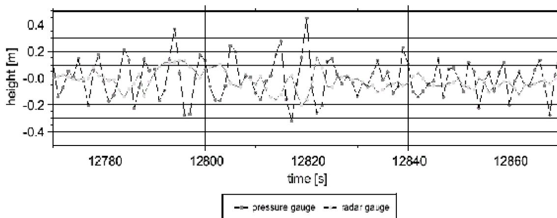
**Figure 4.** Comparison of 1-Hz measurements of pressure and radar gauge.
