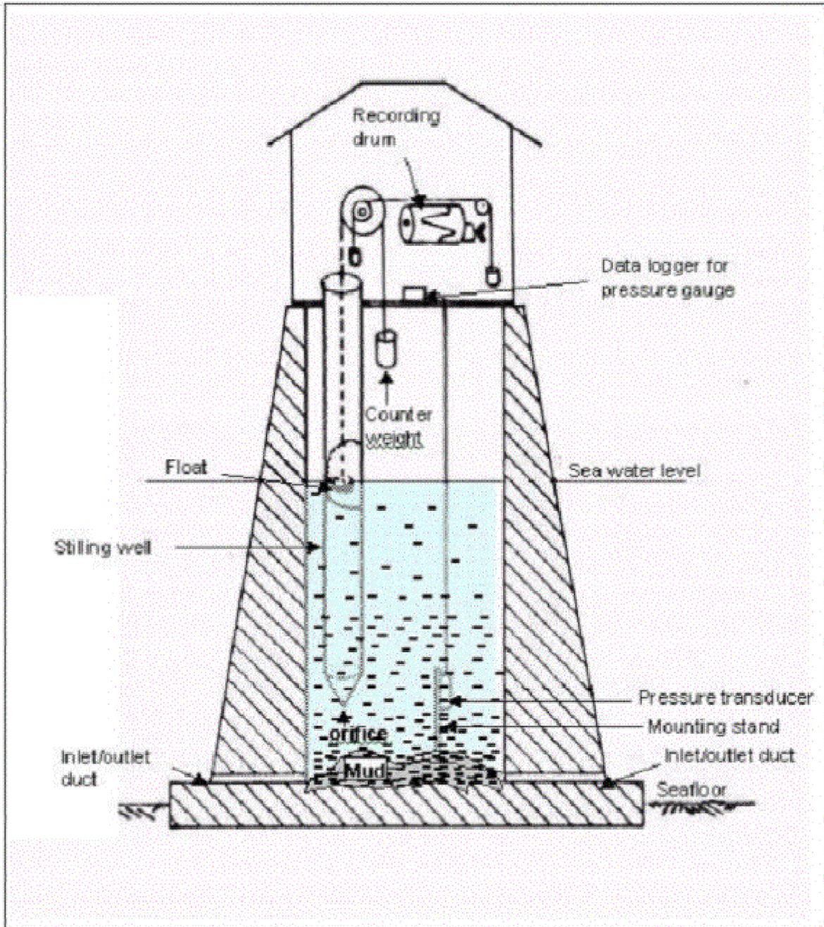
**Figure 5.** Concrete well, at Apollo Bundar, Bombay, which is hydraulically connected to the sea via two tubular ducts at its bottom portion and trapped sediments (After Joseph, 1996).
