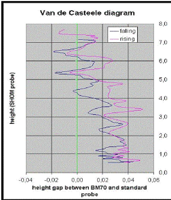
**Figure 4.** Comparison of the SHOM probe and BM70 radar (in a PVC tube) plots.
