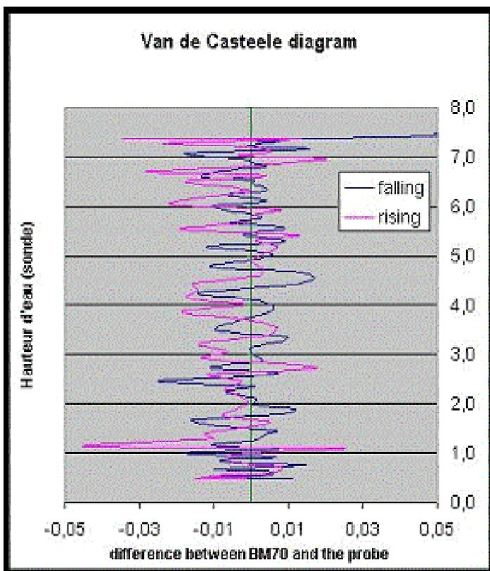
**Figure 5.** Comparison of the SHOM probe and BM70 radar (in a stainless-steel stilling well) plots.
