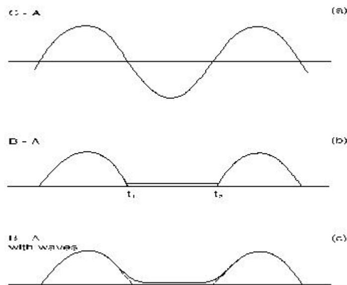
**Figure 3.** The principle of the "triple point" method: (a) the full tidal curve "C" with the atmospheric pressure signal "A" removed; (b) the half-tide signal "B" with the atmospheric pressure signal removed; (c) as (b) but showing the effect of waves on the half-tide curve.
