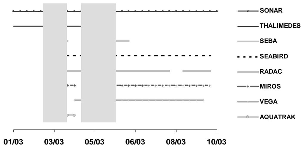
**Figure 4.** Periods of functioning of the gauges and periods of intercomparison (inside the grey boxes).
