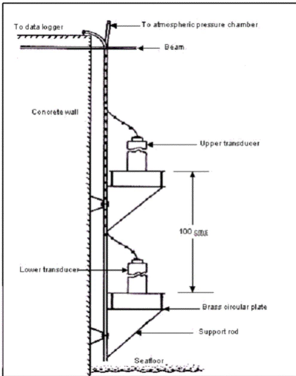
**Figure 7.** Schematic of dual pressure gauge system deployment in Zuari estuary, Goa, for automated *in situ* estimation of effective density of water and effective-density-compensated measurement of sea level (After Joseph, 1996).
