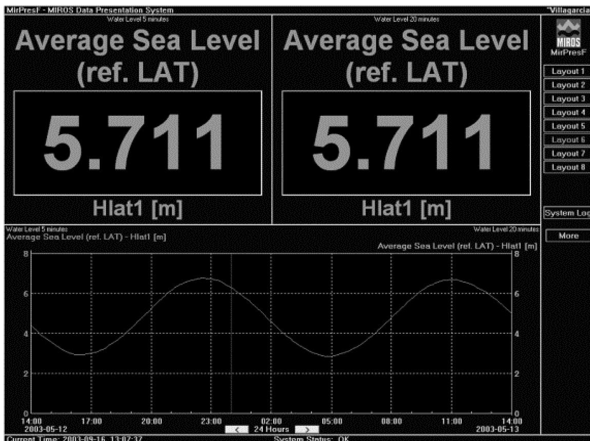
**Figure 4.** Simple and clear layout (gray-scale bitmap) showing two singles and one history graph.
