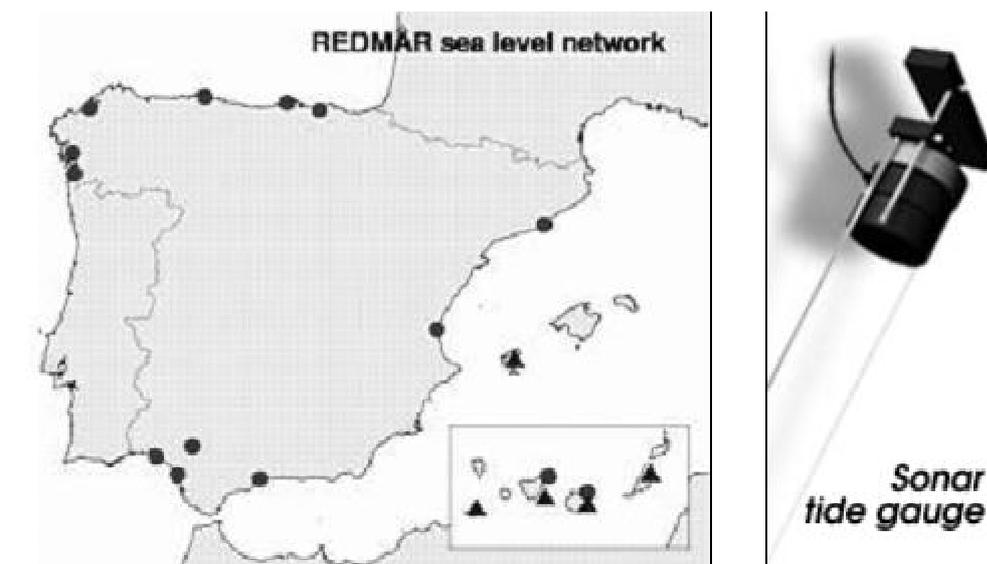
**Figure 1.** Left: the REDMAR stations (circles: acoustic sensors, triangles: pressure sensors); right: sonar transducer.
