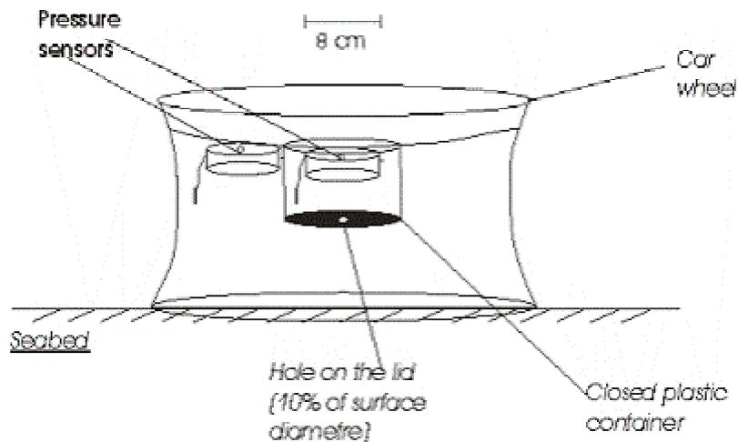
**Figure 6.** A simple wave damper for electronic pressure sensors.
