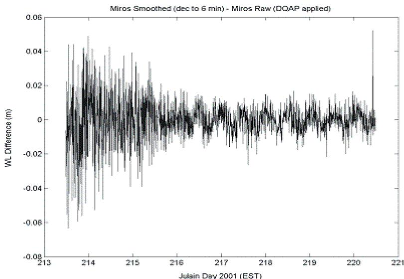
**Figure 2.** Difference time series of two different smoothing processes (Miros recursive minus NWLOP DQAP) operating on a single data set from a Miros SM094.
