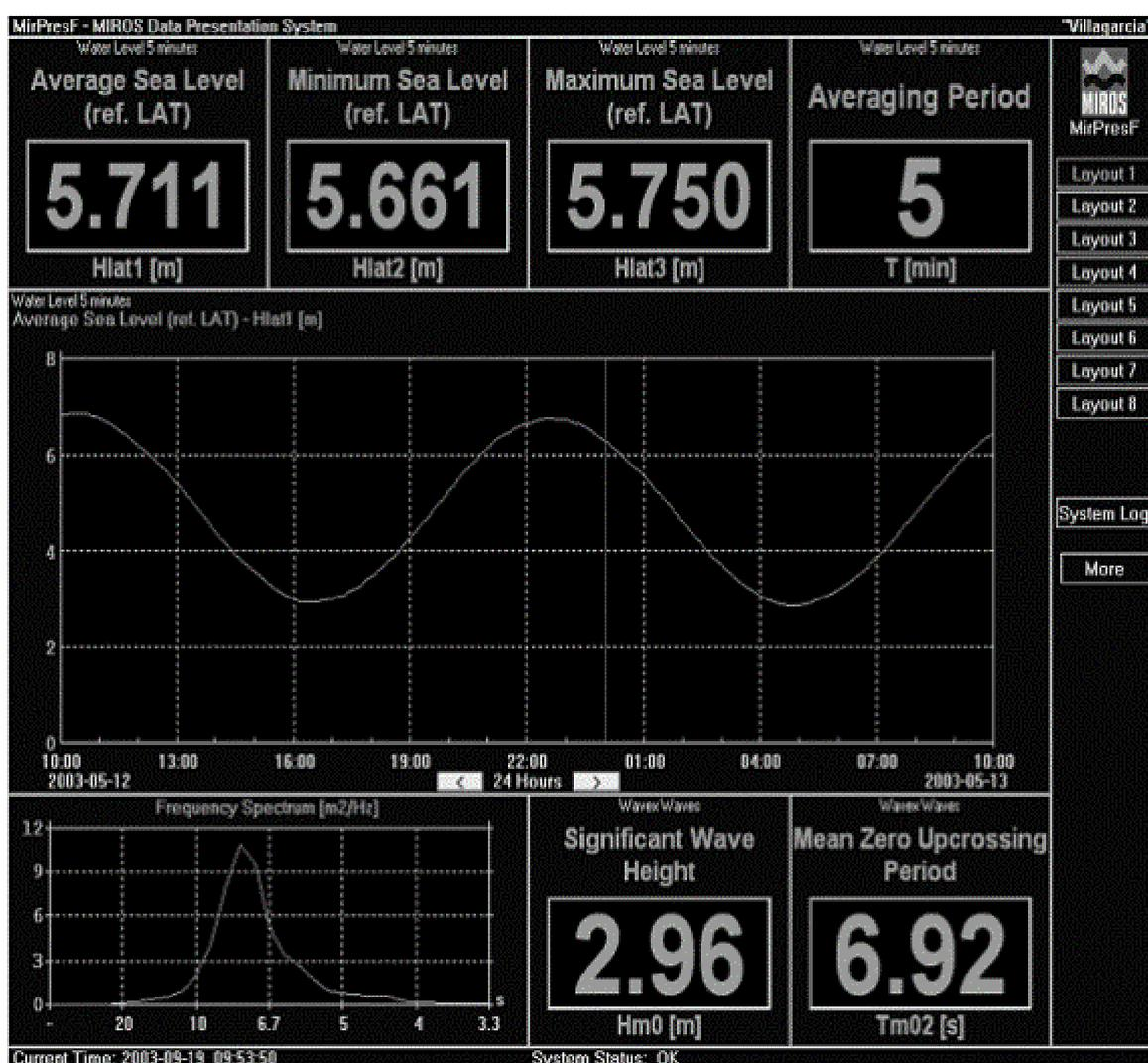
**Figure 3.** Typical display (gray-scale bitmap) of the display system module.
