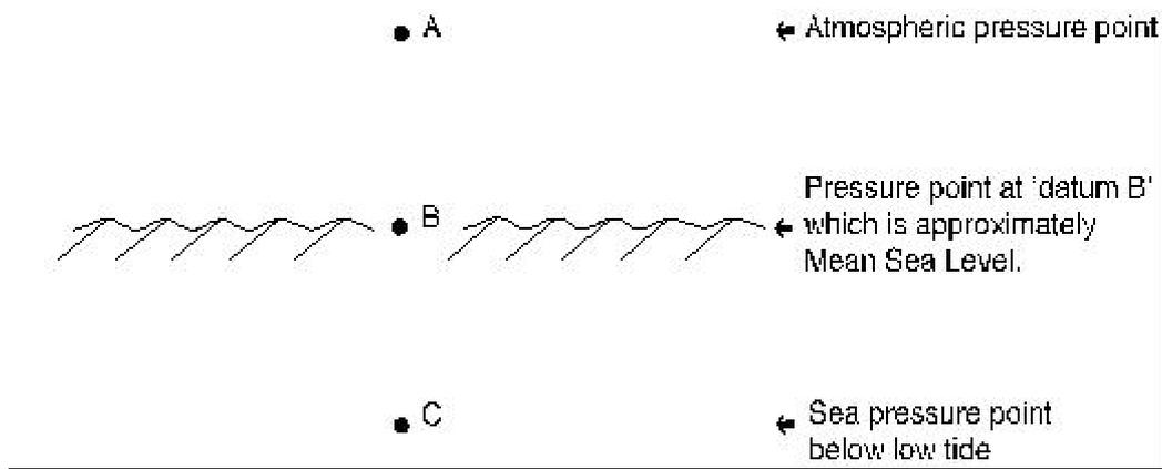
**Figure 2.** Schematic of a pressure gauge set-up using three pressure transducers. Note that all three transducers can drift, as can the ocean itself.
