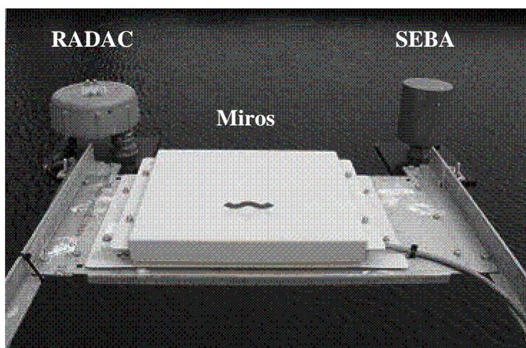
**Figure 3.** Picture of three of the radar sensors installed at the test site.
