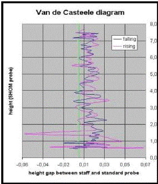
**Figure 2.** Comparison of the SHOM probe (in a stilling well) and the tide staff plots.
