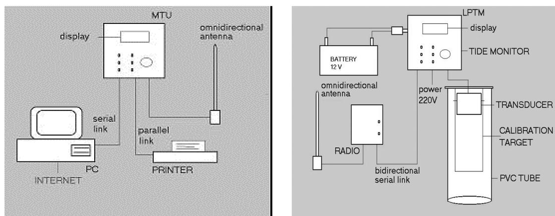
**Figure 2.** Elements of a typical SRD station with radio link (left: elements at the harbour office; right: elements at the pier, all of them, except the tube with the transducer, are inside a small hut).
