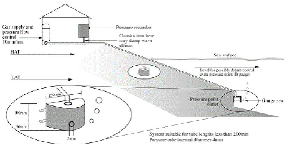
**Figure 1.** A typical bubbler gauge installation (From Pugh, 2004, copyright reserved).
