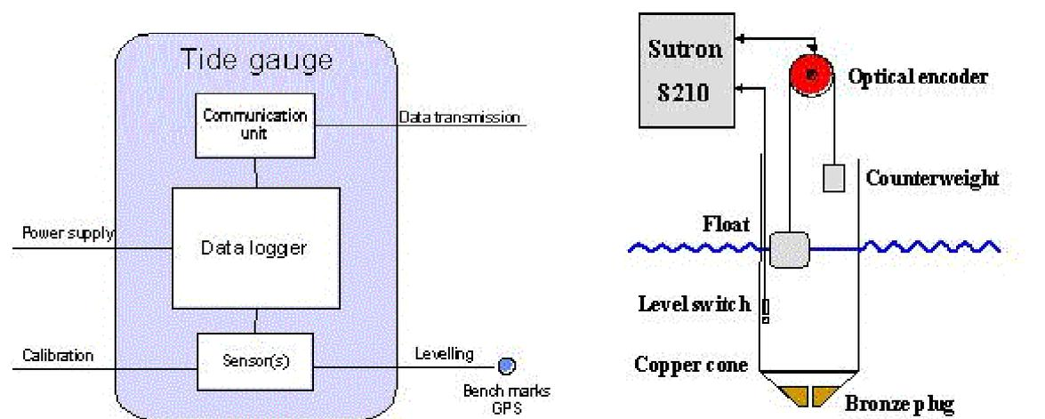
**Figure 2.** Schematic representation of the tide gauge used in the Norwegian tide gauge network.
