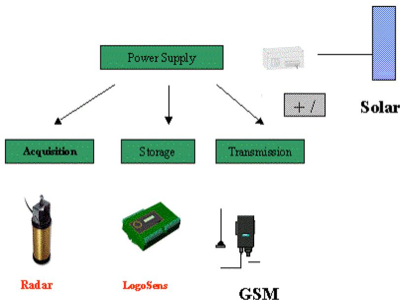
**Figure 1.** Representation of the Kalesto system powered by solar panel and local battery.
