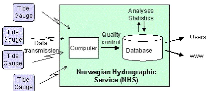
**Figure 1.** Schematic representation of the Norwegian tide gauge network.
