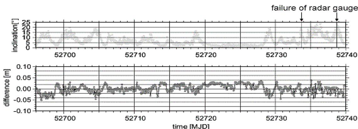
**Figure 6.** Difference of pressure and radar gauge and extreme inclination of the buoy.
