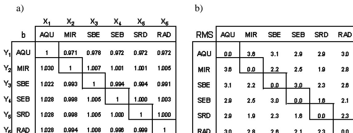
**Figure 5.** Results of the intercomparison of the different gauges in March. Slope of the linear regression (a) (dimensionless) and RMS (b) (results in centimetres).
