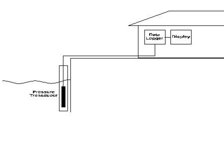
**Figure 1.** Schematic of the "transducer in the sea" pressure system.
