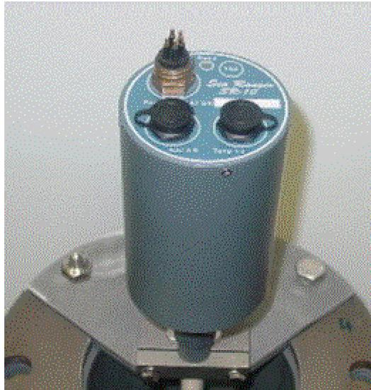
**Figure 2.** The Sea Ranger acoustic transducer installed over its sounding tube.
