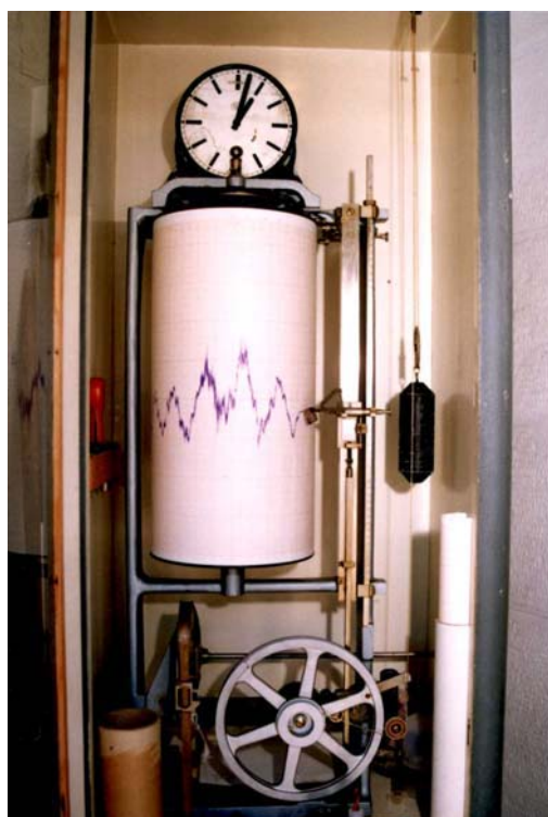
Fig. 2 Mechanical tide-gauge A. Ott – Kempten at Split.
