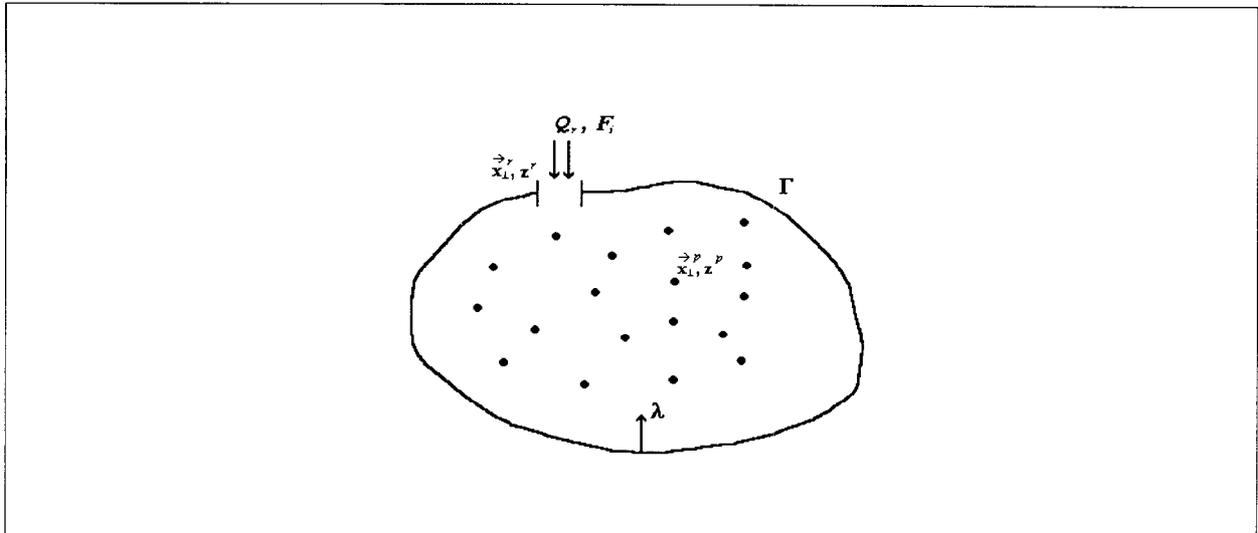
FIGURE 1. Variables and vectors. Dots indicate places where the concentrations of  $i$ th isotope were measured.
