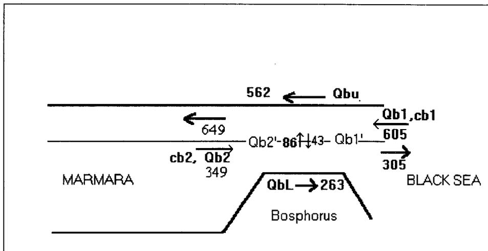
FIGURE 4. Water fluxes (km<sup>3</sup>/y) Bosphorus Strait (after Özsoy et al., 1995).
