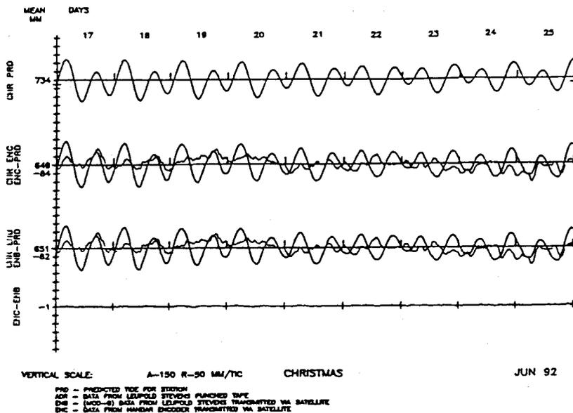
Figure 5. Nine-day time section showing data, residuals, and differences for near-real time data transmitted by the Handar DCP via satellite and received at UH.
