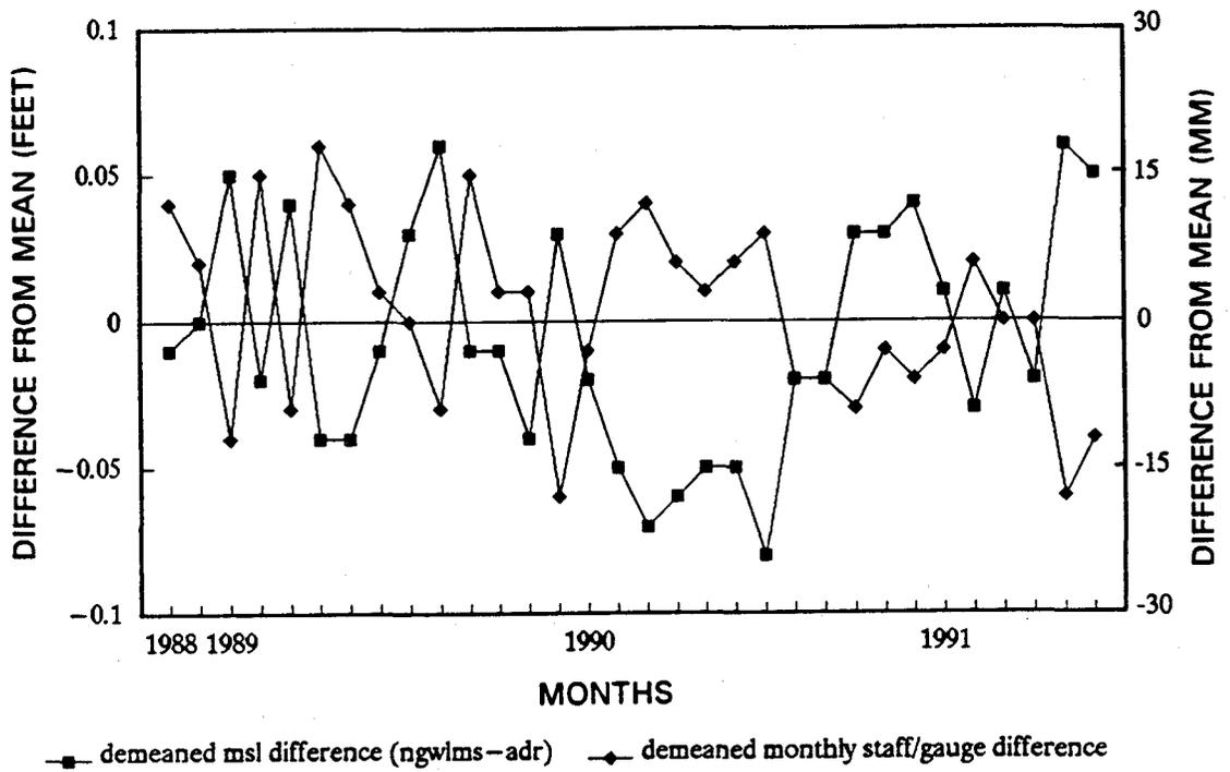
Figure 3. The difference between NGWLMS and ADR monthly means at Monterey, California plotted on the same graph with monthly staff/gauge differences.
