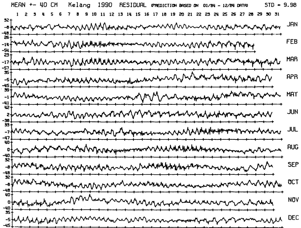
Figure 9b. Hourly residuals displaying shallow water, non-linear fluctuations due to the inability of the tidal analysis to resolve these higher frequency tidal components. These high-quality data are from a digital float and well gauge that samples every 10-seconds with 50-second averages, which in turn are decimated to hourly with a five-point filter.
