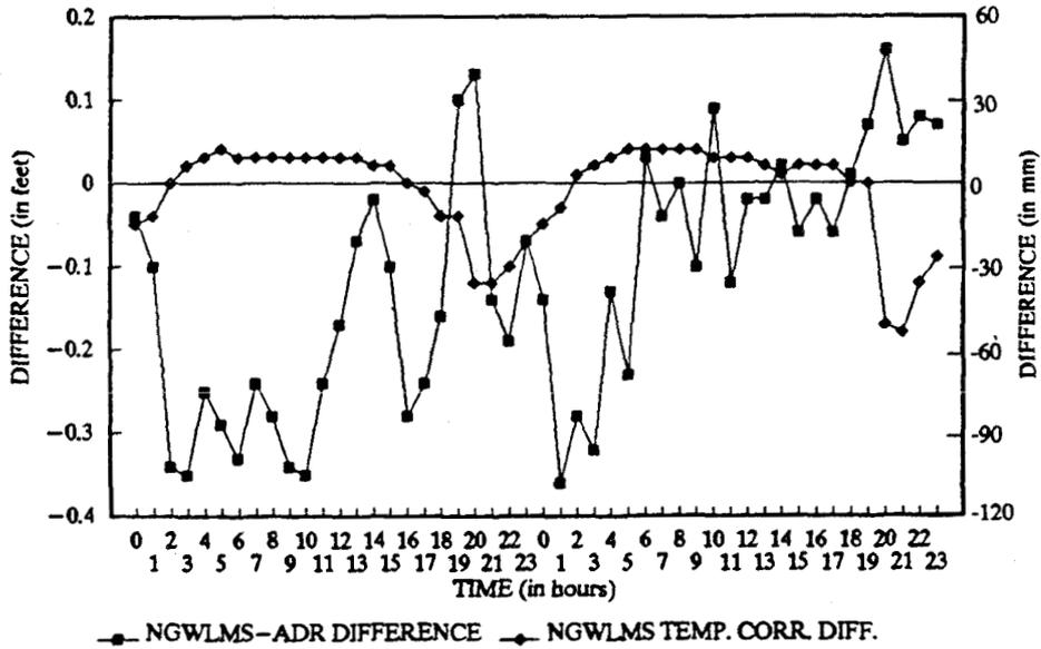
Figure 2. The hourly height differences between the NGWLMS and the ADR for two different two-day periods from the Scripps pier. (The NGWLMS values are not corrected for a temperature effect.) Also shown in the two plots is the first-order correction that would be made to the NGWLMS water level based on the difference in temperature at the two thermistors on the sounding tube.
