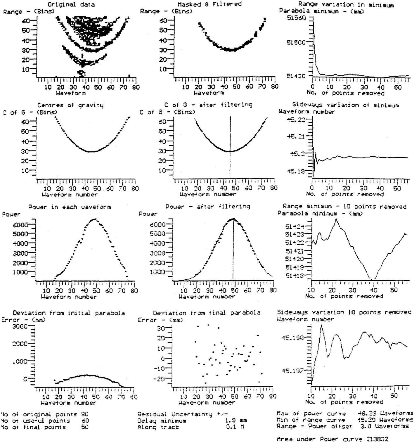
Fig. 2 The plots above illustrate the filtering, bad data rejection and curve fitting that is applied to determine the delay minimum from raw altimetry data collected in the low resolution "Ice Mode".
