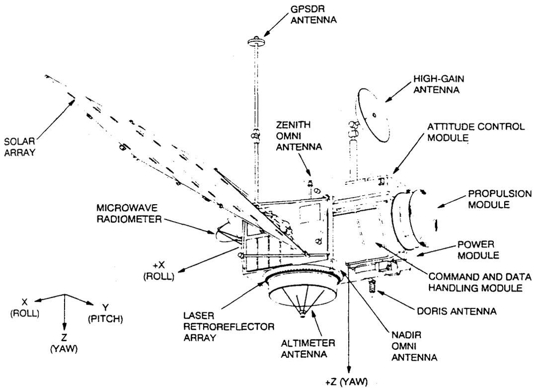
Figure 2 : The TOPEX / POSEIDON Satellite configuration (from JPL publication 92-9)
