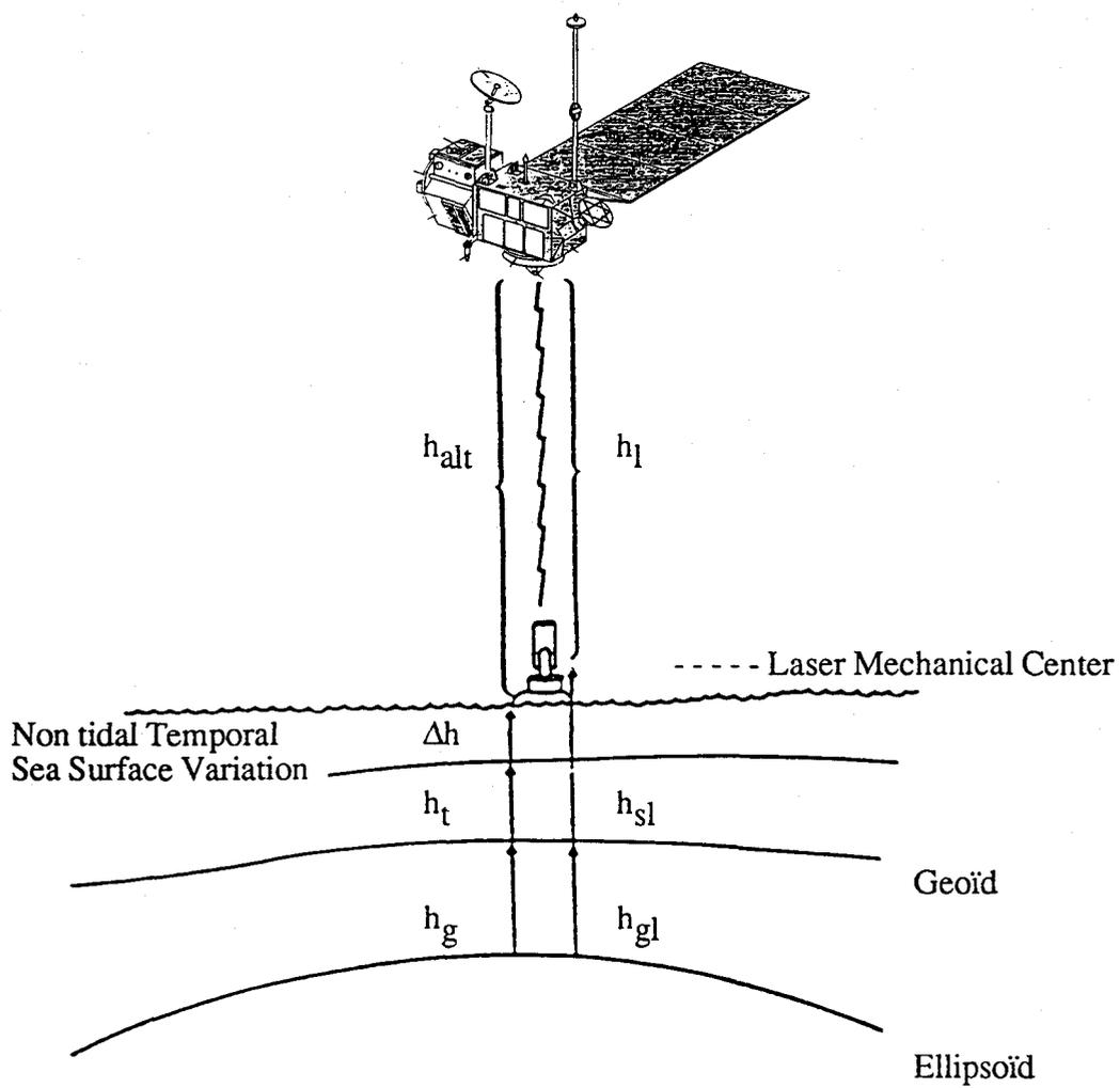
Figure 3: Calibration Geometry using laser station nearby the calibration site.
