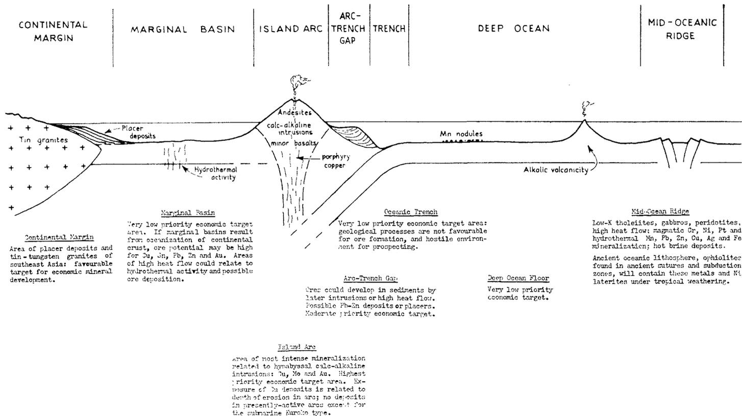
Figure 3. Economic significance of the various plate tectonic elements in the marine domain.
