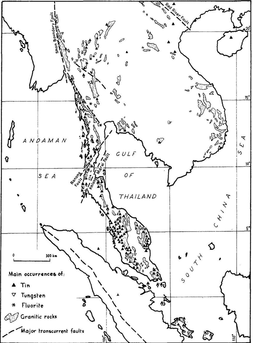
Figure 4. Distribution of tin, tungsten and fluorite mineralization in relation to granitic rocks in southeast Asia (from Mitchell and Garson, 1972).
