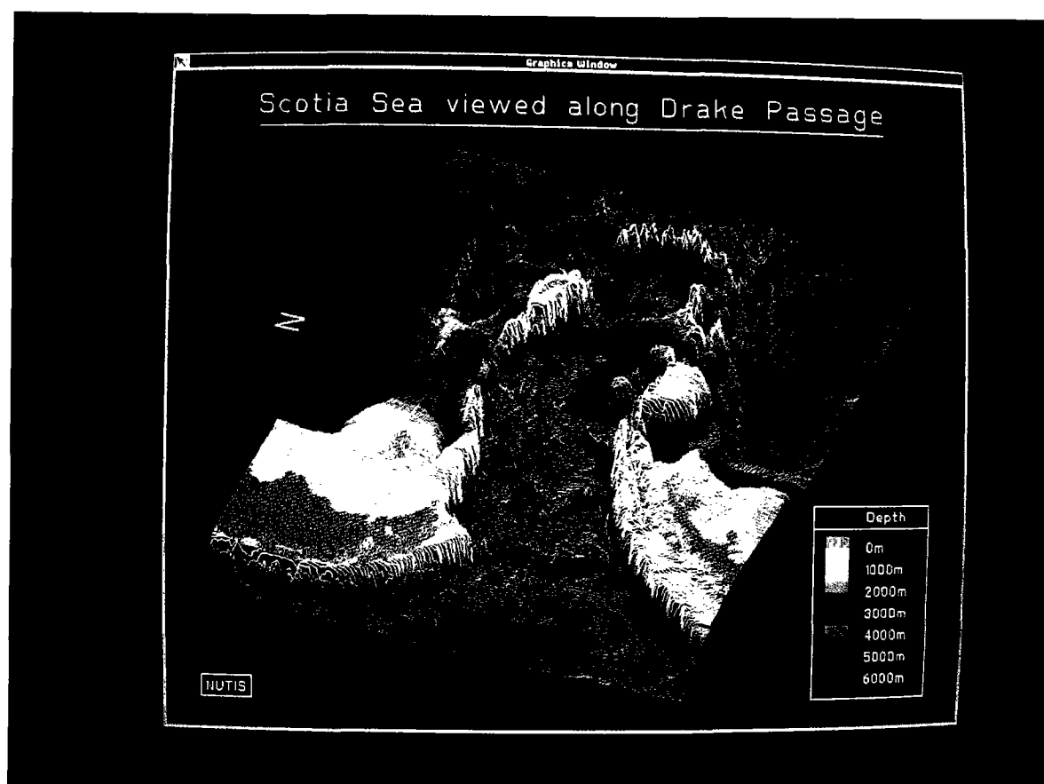
Figure 3 Digitization of the contours of the 5th edition of GEBCO and subsequent generation of digital terrain models enables the GEBCO data set to be manipulated to give different views of the topography. (Courtesy NERC Unit of Thematic Information Services).
