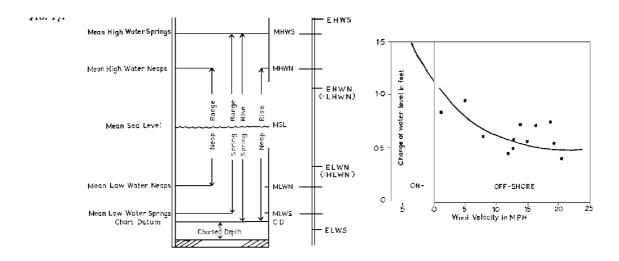
Figure 1. (A) *Left* - The nomenclature of tidal levels for mean springs and neaps, showing the extent of the range and c the rise as related to 'Chart Datum'. Extreme levels for springs and neaps are shown in the separate column. (B) *Right* - The effect of onshore and offshore winds in raising and lowering the water level of predicted tides.
