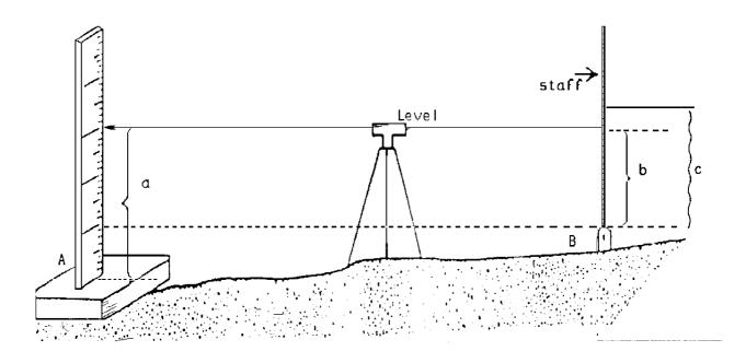
Figure 4. Beach profiling with the aid of a surveyor's level.
