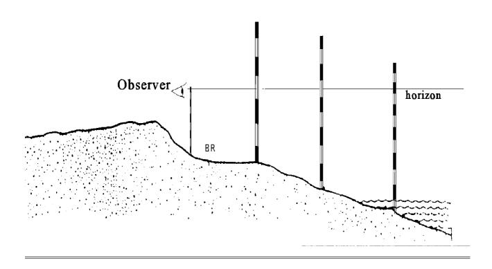
Figure 5. Beach profiling by an observer sighting the horizon from a fixed point.
