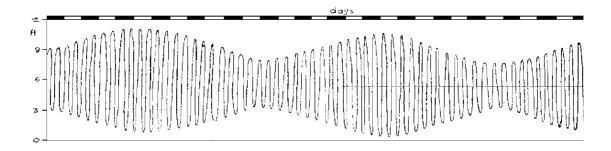
Figure 2. The tidal curve for semidiurnal tides with two sets of springs and two of neaps, over a period of one month.
