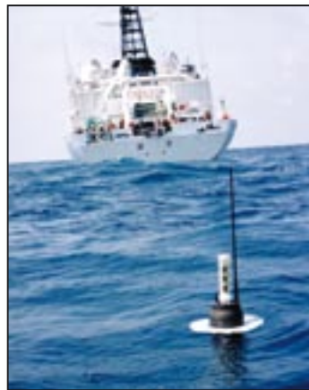
An Argo float just after launch from the Japanese Coast Guard vessel Takuyo .
