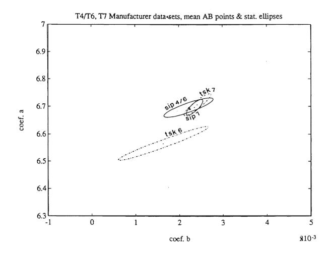
Figure 11 Mean Sippican and TSK T-7 and T-4/T-6 *AB* points and their two-standard-error-of-the-mean ellipses on the *a-b* plane (95% confidence level; same scale as Fig. 9; see Table 2 for detailed information).
