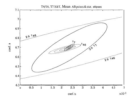
Figure 7 Standard deviation ellipses on the a-b plane of the T-4/T-6 and T-7 mean A, B coefficients (the b scale is 3 times smaller than in Fig. 5): i) The outside dashed ellipses and the large solid ellipse are respectively the T-4/T-6 and T-7 'individual' 2-standard deviation ellipses of Figs. 5 and 6. ii) The small intersecting dashed and solid ellipses are the 1, 2, 3 standard-error-of-the-mean ellipses for, respectively, the T-4/T-6 and the T-7 ab points.
