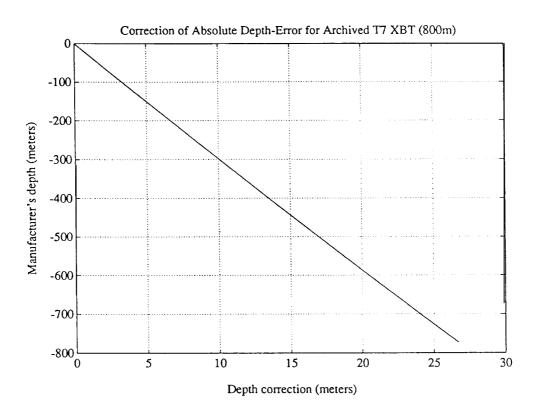
Figure A2.1: Full correction of the manufacturer's depth (depth-time equation's coefficients: a = 6.472, b = 0.00216), as a function of that depth. The new depth equation is the T-4/T-6/T-7 reference depth-time equation (coefficients A = 6.691, B = 0.00225).
