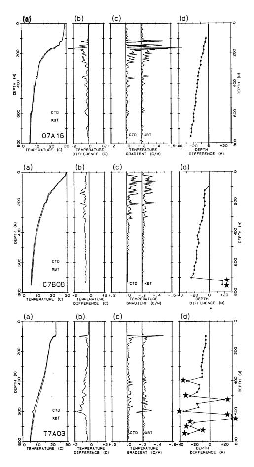
Figure 4. Three typical examples of comparison data: 07A16, C7B08 and T7A03 (see Table 1 for details): (a) CTD (thin line) and XBT (thick line) temperature profiles; (b) profile of the temperature difference (XBT minus CTD); (c) CTD and XBT temperature gradient profiles (XBT temperature gradient profiles are offset by  $-0.2^{\circ}$ C/m); (d) detected XBT depth-errors. Depth-errors marked by \* are considered erroneous and discarded.
