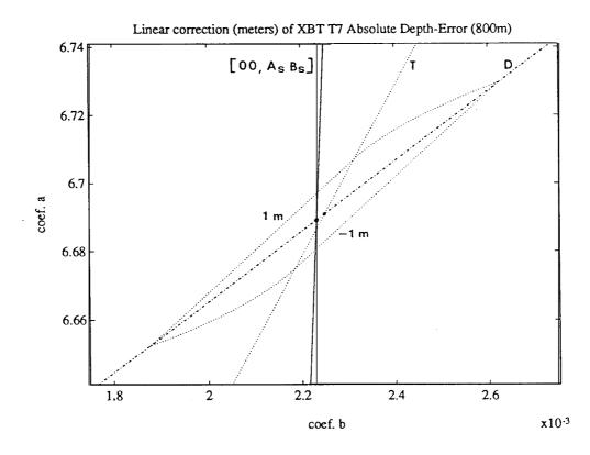
Figure A2.2: Determination of a 'best' linear approximation's coefficient to correct the manufacturer's depth to the new reference depth (*AB* point \*). On the *a-b* plane, the 'best' linear correction coefficient 1 is found at the intersection (o) of the [00 ab] full line locus of the linear corrections, with the discontinuity line (dash-dotted *D* line) locus of the minimum depth-errors. The dotted lines are the  $\pm 1$ m maximum absolute depth-error isolines and the transfer line (7).
