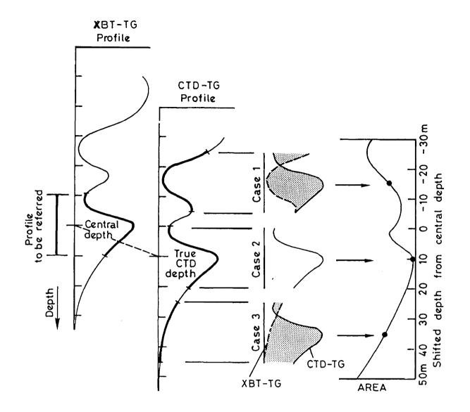
Figure 3. Explanatory picture of the detection method adopted to determine the XBT depth-error (adapted from Hanawa and Yasuda, 1992). See section 3. I .1, *step* 4, in the text for details. In this figure, only three examples are shown. Since the area has its minimum value in Case 2, its shifted CTD central depth is the actual depth of the reference central XBT point, and its depth-shift (+10m) is regarded as the depth correction of the XBT data.
