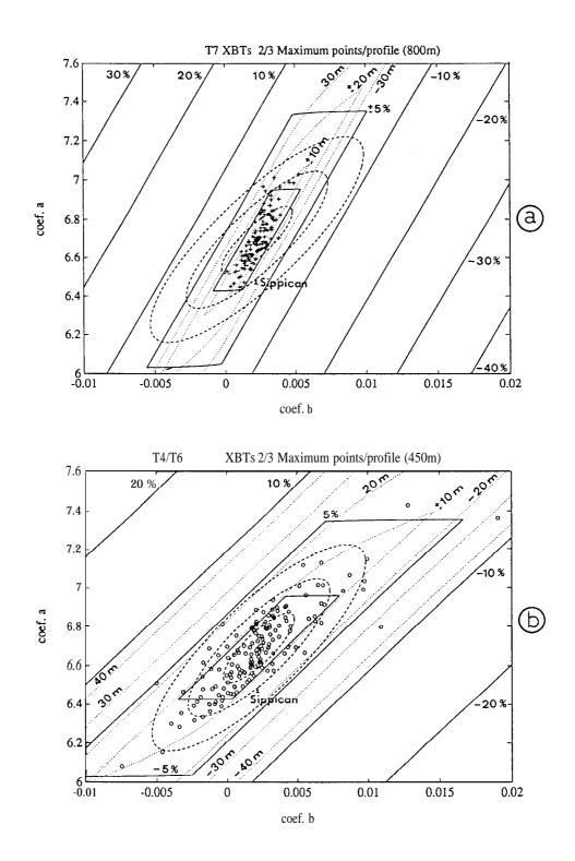
Figure 8. T-7 (upper) and T-4/T-6 (lower) data sets presented on their respective *a-b* plane of the new T-4/T-6/T-7 equation (800m or 450m maximum depth; same scales as Fig. 6). The reference  $A B_{467}$  point ( $A_{467} = 6.691$ ,  $B_{467} = 0.00225$ ; marked by an \*) is at the center of the ellipses.
