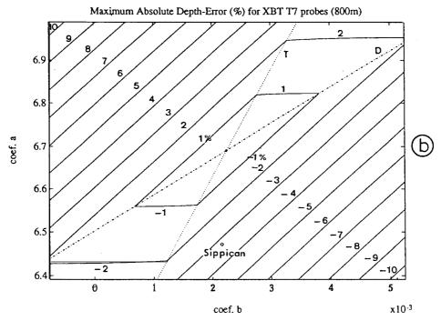
Figure A1.4: Maximum absolute depth-error expressed as a relative error on the same a-b planes as in Fig. A1.2: *i*) The full lines are absolute maximum depth-error isolines, expressed in percentage of the depth at which the error occurs.
