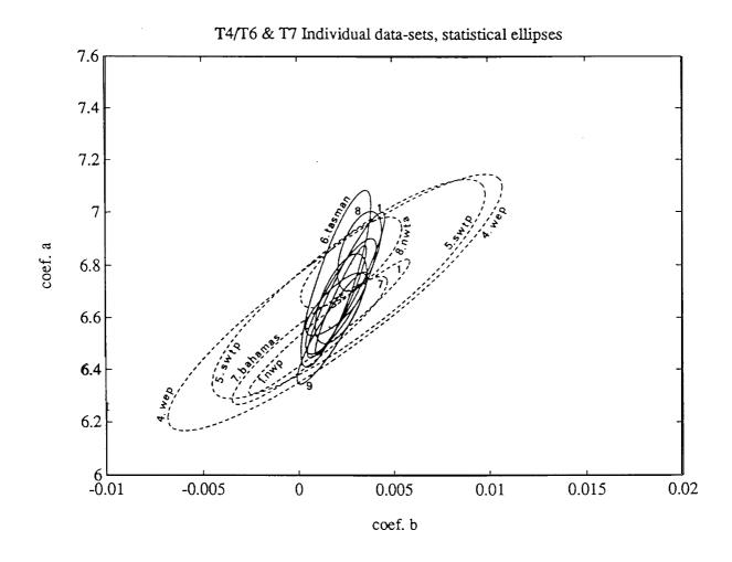
Figure 13 Individual regional 2-standard deviation ellipses on the a-b plane (95% confidence level; same scale as Fig. 6; see Fig. 1 and Table 1 for the location of the regions). The full and the dashed ellipses are, respectively, the T-7 and the T-4/T-6 individual regional ellipses. For clarity, in the central group, some ellipses are referred to by their region number only.
