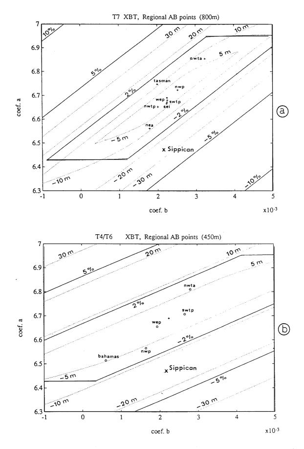
**Figure 12** Regional *AB* points on the new  $AB_{467}$  (marked by an \*) reference planes of Fig. 8 (T-7 800m and T-4/T-6 450m maximum depth-error planes), but with the scales of Figs. 9 and 11.
