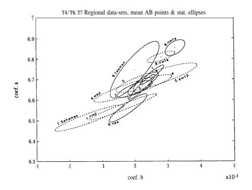
Figure 9 Mean regional two-standard-error-of the-mean ellipses on the *a-b* plane(95% confidence level); see Fig. 1 and Table 1 for the location of the regions). The full and the dashed ellipses are, respectively, the T-7 and the T-4/T-6 mean regional ellipses. For clarity, in the medium group some ellipses are referred to by their region number only.
