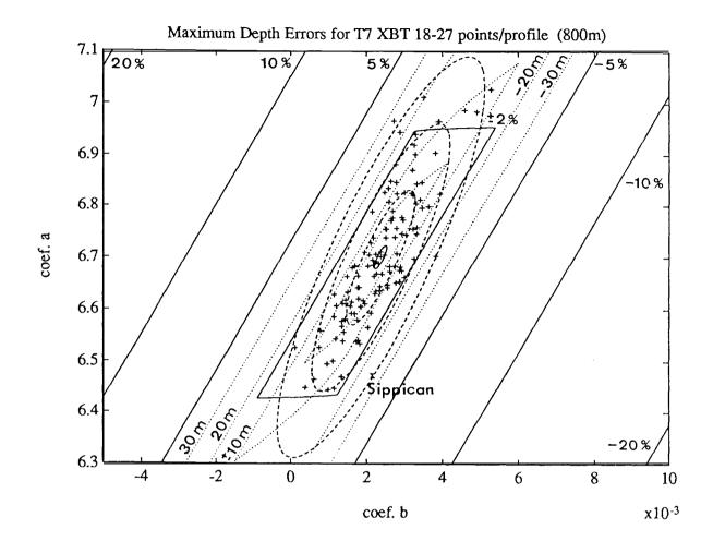
*Figure 5, T-7 XBT probes on the a-b* plane of the new T-7 equation (Eq. 7, reference  $AB_7$  point marked by an \* at the center of the ellipses:  $A_7 = 6.701$ ,  $B_7 = 0.00238$ , see Appendix 1 and Table 1 for full explanations):
