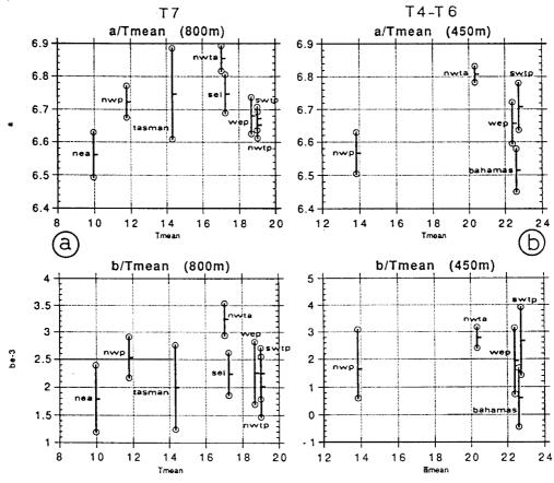
Figure 10 The mean *A*, *B* coefficients and the two-standard-error-of-the-mean bars for the different regions of the XBT-CTD experiment are plotted against the mean temperature of the water between the surface and the maximum depth reached by the probe type (a: 800m for T-7, b: 450m for T-4/T-6). See Fig. 1 for the location of the regions. The mean temperature has been computed using the Levitus (1982) T-S data of Fig. 2.
