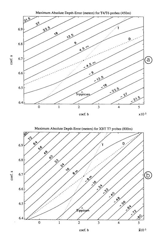
Figure A1.2: Maximum absolute depth-error on the *a-b* plane (centred on the  $AB_{467}$  point \* of the new reference T-4/T-6/T-7 depth-time equation:  $A_{467} = 6.691$  and  $B_{467} = 0.00225$ ), for T-4/T-6 and T-7 probes:
