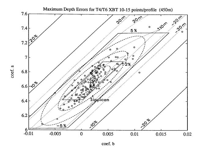
Figure 6. T-4/T-6 XBT probes on the *a-b* plane of the new T-4/T-6 equation (Eq. 8, reference  $AB_{46}$  point marked by an \* at the center of the ellipses:  $A_{46} = 6.683$ ,  $B_{46} = 0.00215$ ), (the scales of that figure are twice the scales of Fig. 5, therefore the area shown is 4 times greater):
