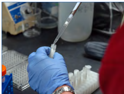
Figure 5. Addition of lysis buffer to cryovial with filter.
