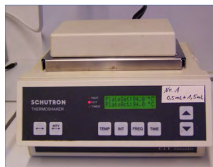
Figure 3. Thermoheater for denaturation of the labelled RNA.
