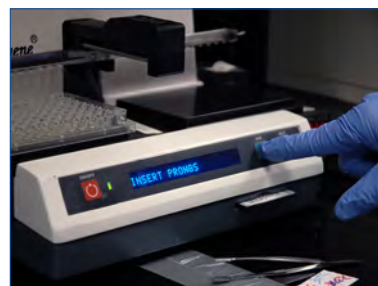
Figure 9. Processor being started after plate is positioned on heater base.
