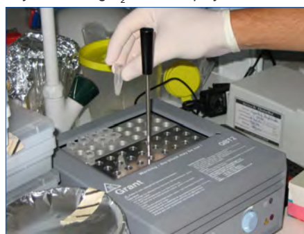
Figure 6. Samples in a thermal block at 55 °C.
