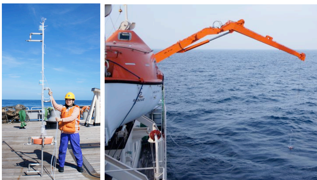
Fig.1 The profiling buoy and the aspect of the measurement by use of ship crane.
