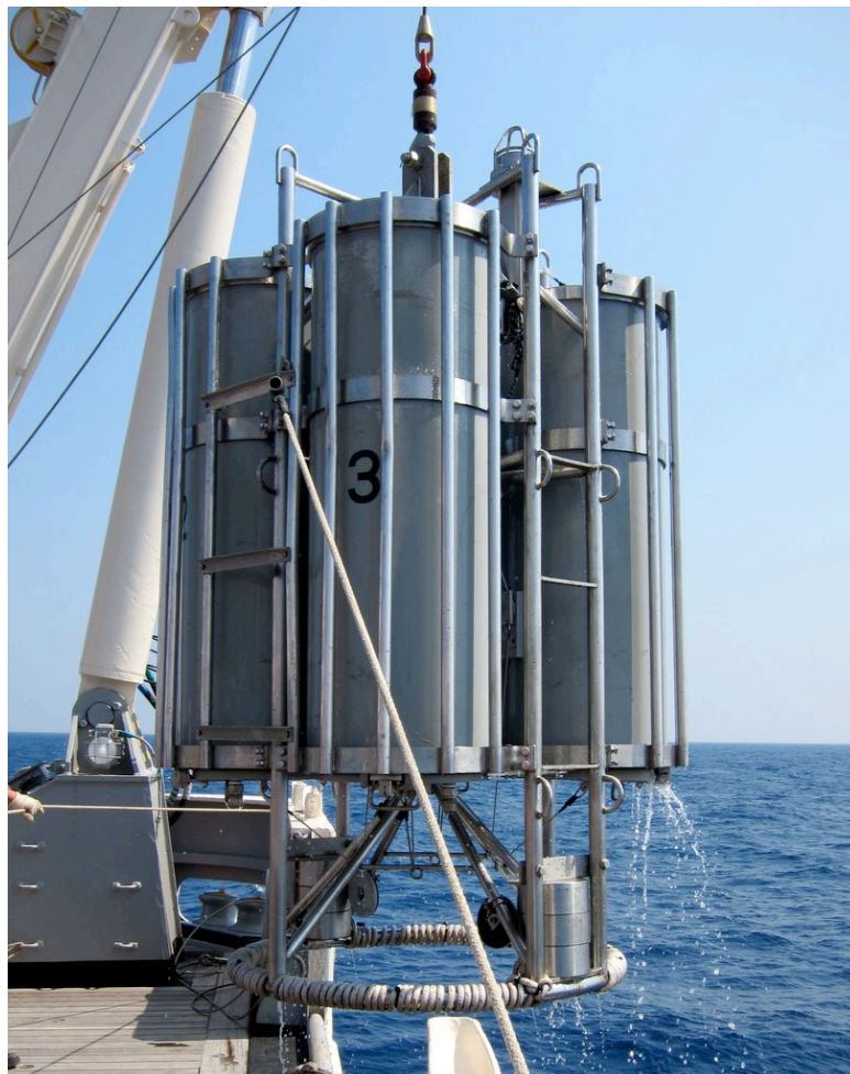
Fig. 1 Photograph of the large-volume water sampler used in the KH-12-4 cruise.
