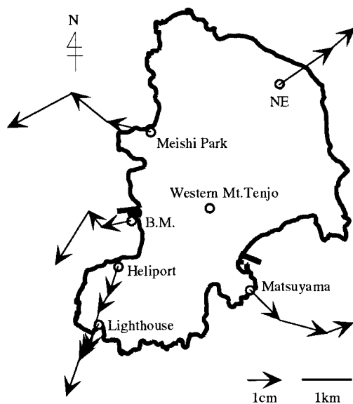
Fig. 10 The results of GPS dense observation at Kozu-shima from Jan., 1997 to Feb., 2000. Western Mt.Tenjo is fixed.
