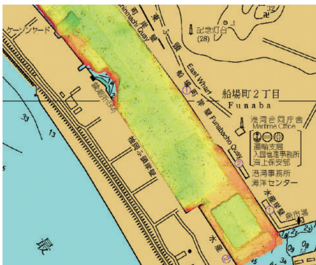
Fig. 6. Trace of dredging on the seabed of Port of Sakata, Yamagata. (Dredging area can be clearly identified). (Map re-drawn from survey results of Sakata-ko, 2019).
