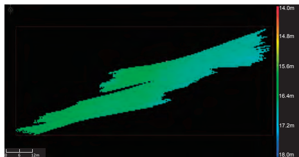
Fig. 9. 0.5 m gridded reference bathymetric data of stationary observation (phase A-3) obtained with SeaBat 8125.
