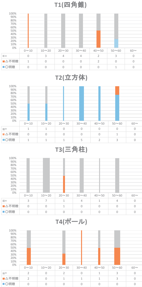
Fig. 15. Verification of feature detecting capability of GeoSwath at target survey (phase F-1). Ratings of feature detection are counted up for each 10-degree beam band. The width of the bars represents the number of samples.
