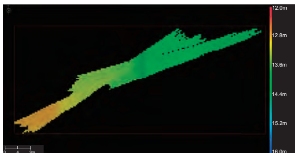
Fig. 5. 0.5 m gridded reference bathymetric data of stationary observation (phase A-1) obtained with SeaBat 8125.
