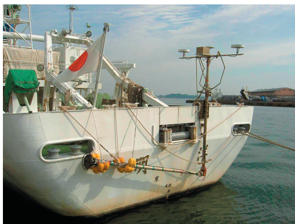
Photo 3. Observation pole installed on the bulwark at the stern.
