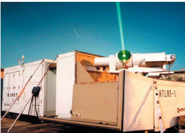
Photo 4. Hydrographic department Transportable Laser Ranging Station (HTLRS).
