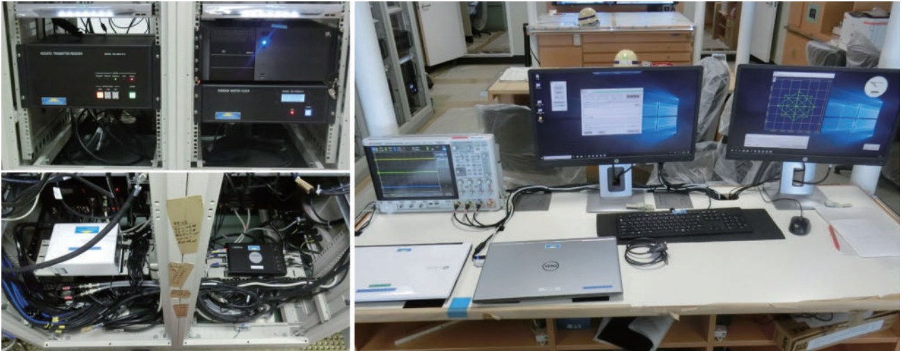
Photo 6. Control and recording devices for the seafloor geodetic observation system installed in the laboratory of S/V Heiyo. (Left upper) Each device of the control unit. (Left lower) GNSS receiver. (Right) PCs on the control desk.
