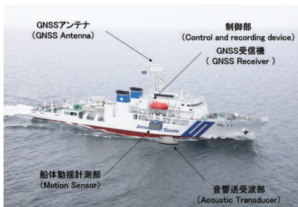
Photo 1. Locations of installed equipment for the GNSS-Acoustic observation on the S/V Heiyo. 写真1. 「平洋」に設置した海底地殻変動観測装置の配置.
