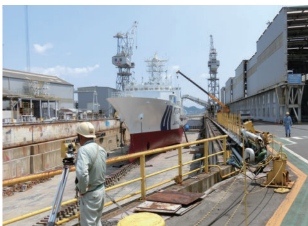
Photo 7. Survey for relative positioning of the GNSS antenna to the acoustic transducer using a total station.
