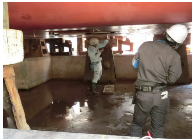
Photo 8. Survey of the height of the acoustic transducer from the bottom of the dock.
