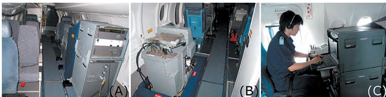
Photo 4. Installation status of CZMIL. (A) Front view of CZMIL. (B) Rear view of CZMIL. (C) The operation situation.
