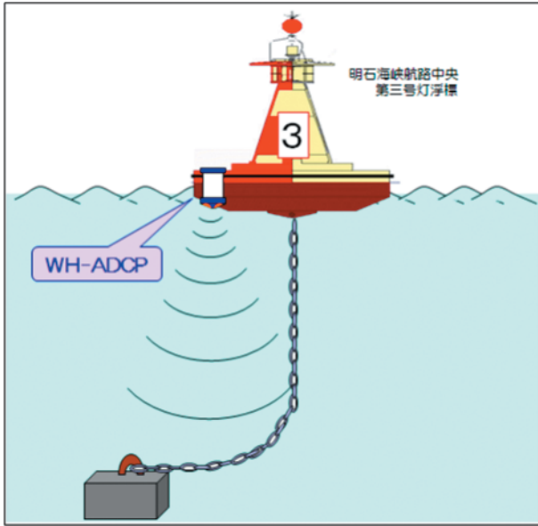
Fig. 2. Schematic image of current observation using an ADCP installed to the floating light. 図 2. 流速計設置状況図.
