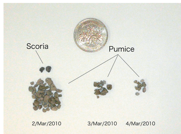
Fig. 5 Volcanic ejecta recovered from the filter of cooling water for engine of “Manbo II”. The great majority of ejecta are pumice, but only two are scoria. Not all ejecta are erupted in the 2010 eruption.
