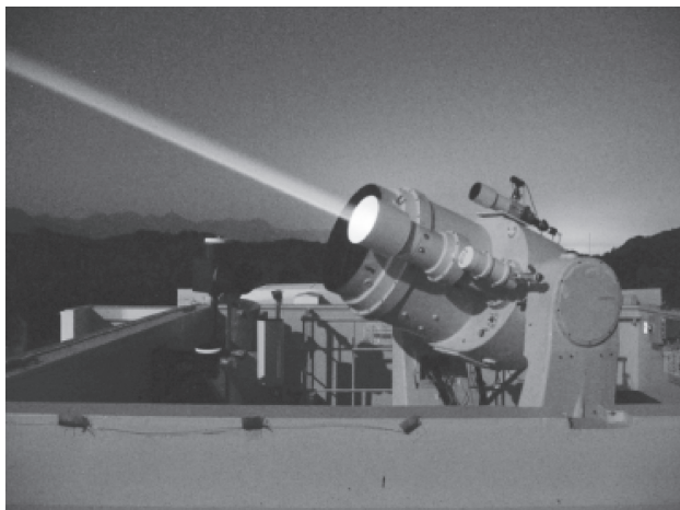
Fig. 1 Satellite Laser Ranging at the Simosato Hydrographic Observatory.
